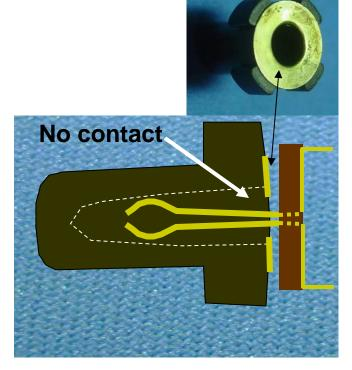
When the door is closed the button "squeezes" the contacts away from the brass contact on the end of the button and the circuit is open: lights out. When the door is open, the button moves forward allowing the contacts to expand and make contact with the brass ring on the button to complete the circuit: lights on!
