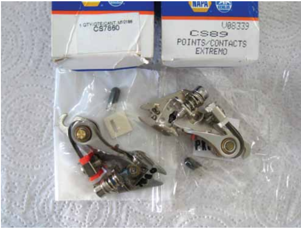
Figure 2: CS7860 with unique felt lubricator pad and CS89. Both are “high performance” 28-32 ounce breaker arm tension. All sets include the grease capsule, but only CS7860 includes the felt pad.
