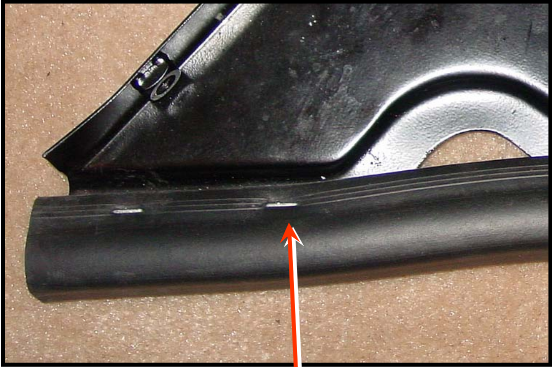
Finished staples top and bottom
