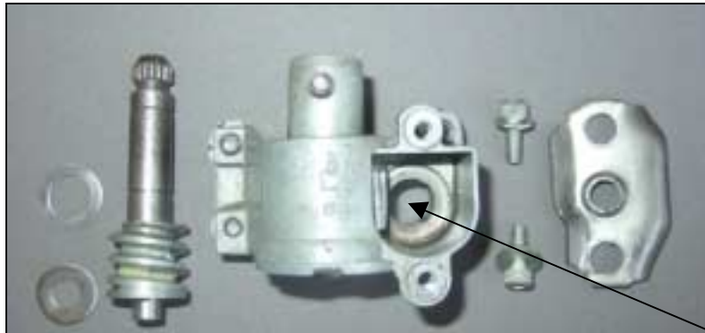
Components of a vent-window regulator
