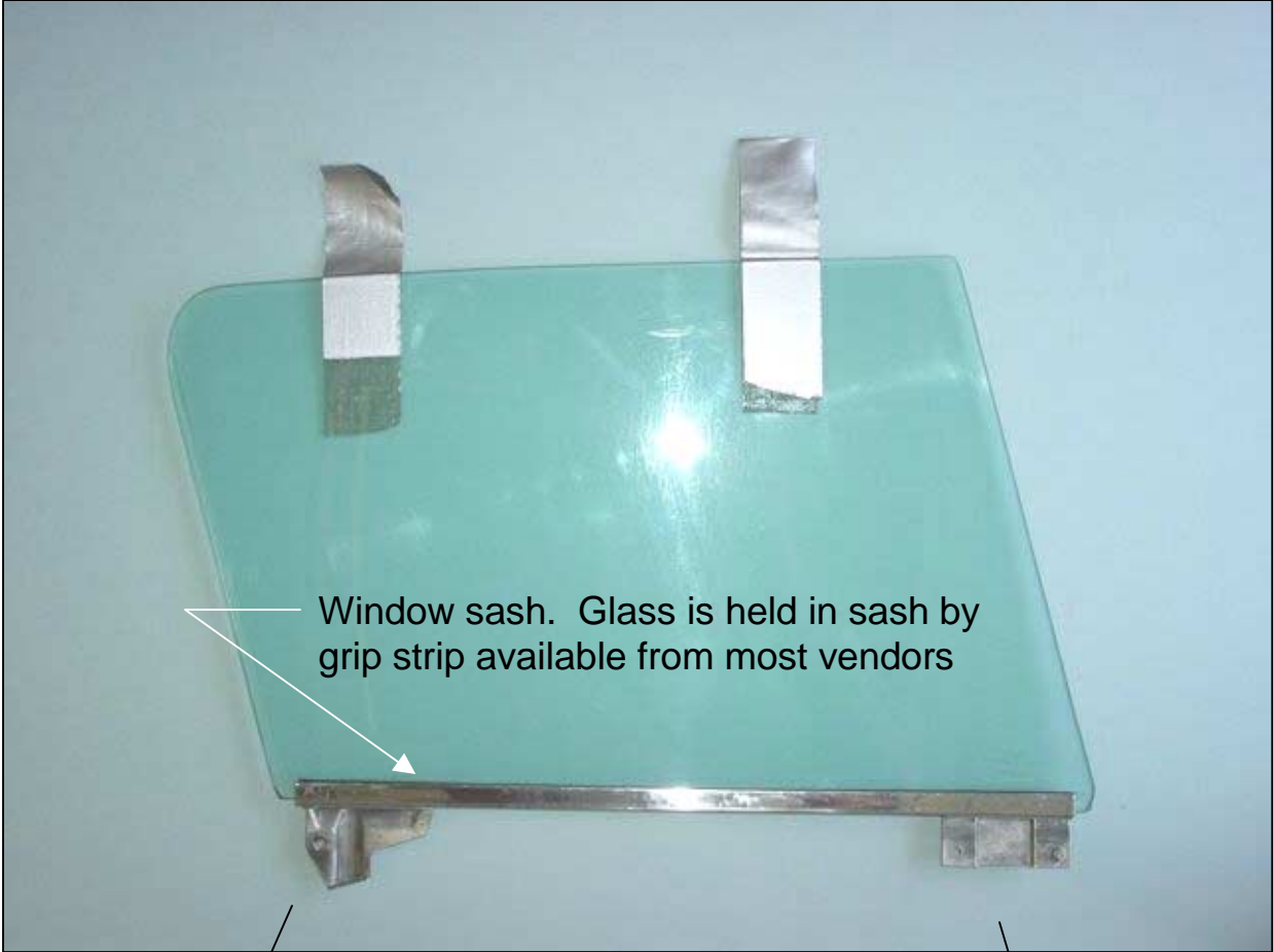
Figure 9: Window sash and mounting studs.
