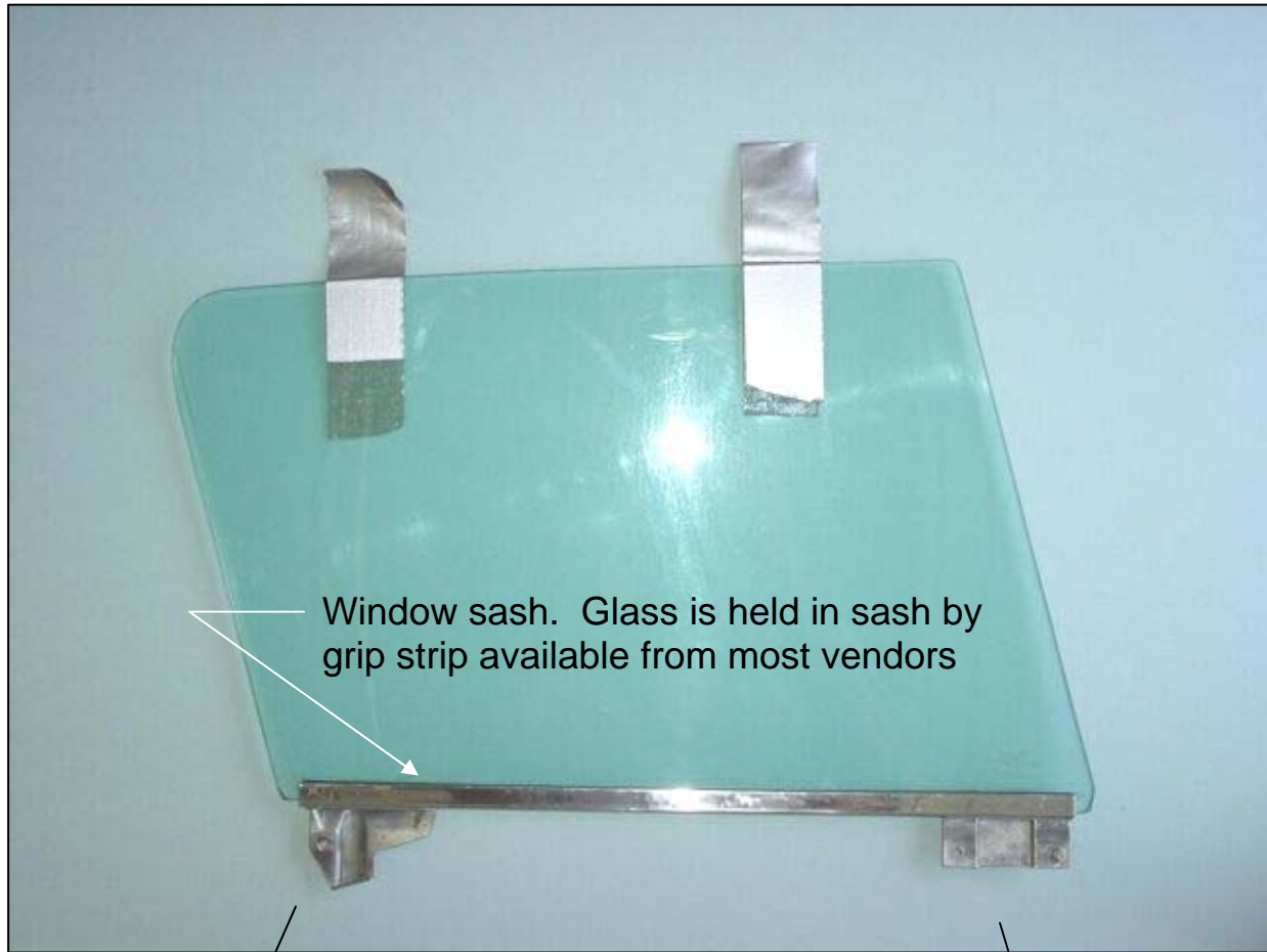
Figure 9: Window sash and mounting studs.
