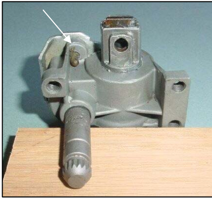
“Front” view of vent-window regulator
