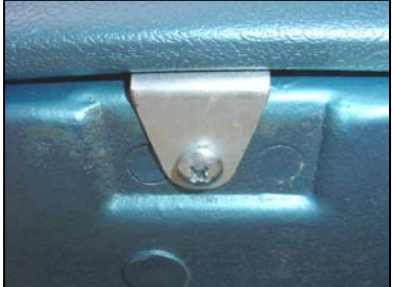
Installed panel clip
