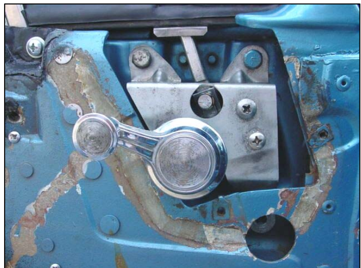
Vent-window regulator installed in door
