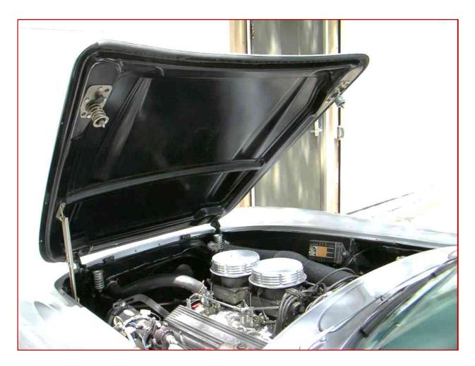
A common fix is to grind or file a notch in the male pins at the "sweet spot" where catches the latch. This way it will catch and hold on to the edge of the circular female latch.
