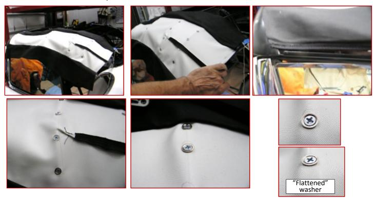
I then measure and attach the rear straps to the #4 bow. This is sometimes (actually always) a trial and error process. Test latching operation and check if straps are snug against the inside of the top. Repeat, test, repeat, until satisfied. Note the error in the AK dimension between #2 and #3 bows. Measure the vinyl from the bow seam up to the top and transfer to the frame.
