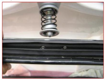
Here it is after frame adjustments. Side windows fit well and doors open and close properly against the weatherstrip. When the vinyl top material goes on, it's important not to stretch it too much as to lose the side window fit, as well as having the top pulling too hard on the windshield frame.
