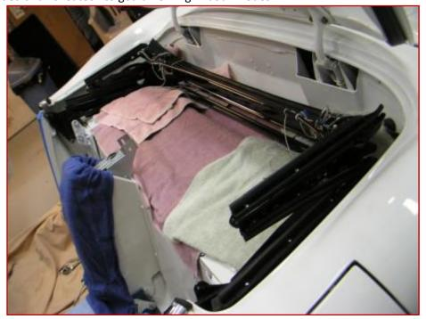
A special concern is to make sure the header clears the deck-lid latch stud too. I always put a protector grommet on that when doing a top and suggest it's always used when raising and lowering a top. You can see it here with some blue tape over it also for added safety.
