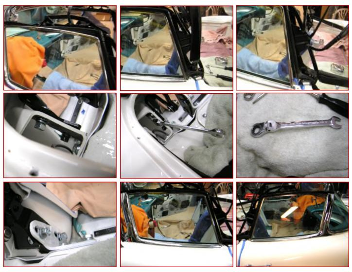
After adjustments for the header and side window fits, it has to be tested to fold down into the well. Sometimes some adjustments are needed and "cheated" to get it working in both modes.
