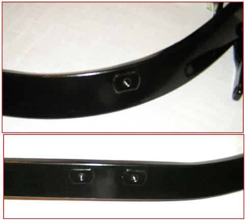
I set up my mill and using a 9/16 end mill bit I shaved the 6 areas to a depth of the thickness of the Tee-nuts. This also will act as a nut-stop when fastening or removing the screws, especially in the future if there is a bit of corrosion in the threads. A thumb press on the flat and it'll lock in on the inside edge of the recess.
