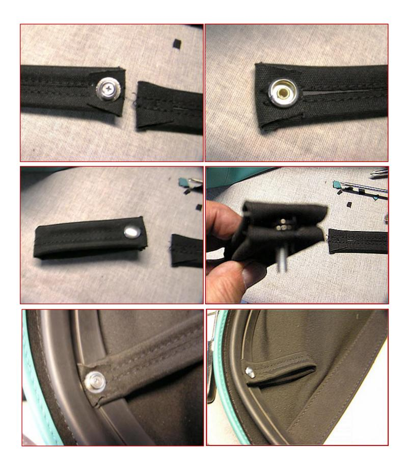
After test fits, I then attach the side flaps to the vertical frames. That center T-nut of the vertical weatherstrip is hard to reach so I tape it to the frame so it doesn't drop. I cut holes in the flap and re-fit the weatherstrips and check the upper rear curves. After the top is done, I release the latches and the weatherstrips again and glue the flap in position, reinstall the weatherstrips and then trim the flaps.
