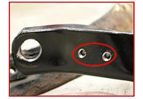
The Tee-nuts are just pressed into the repro bow. They may spin if the screws ever get corroded also. One spun on me when I test fit a swing latch.
