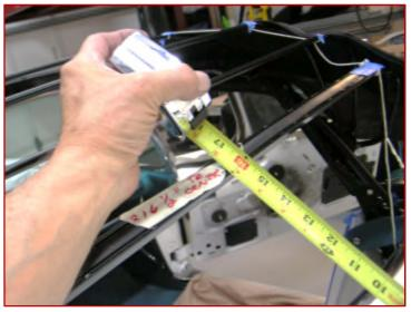
Remove the rear bow and staple the vinyl to the frame while pulling the outer edges taught. Usually 1 3/4" from the pivot bolt to the edge of the side frame piping.
