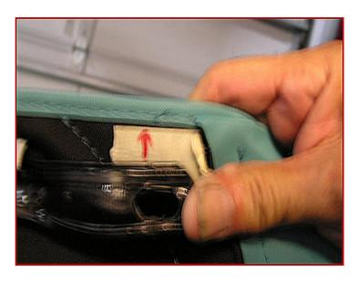
I put some staples to it and test fit the rear bow to ensure the piping looks right at the bottom edges when I stretch the vinyl towards the #4 bow. When stapling, it's important to keep the vinyl aligned along the entire rear bow edge. When satisfied, remove the bow and staple away.
