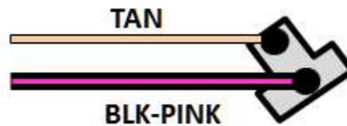
GAS GAUGE (DASH UNIT)
