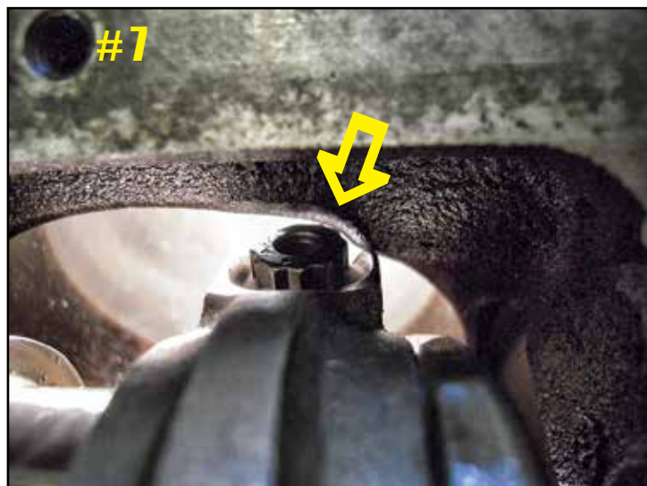
Rod clearance before grinding
