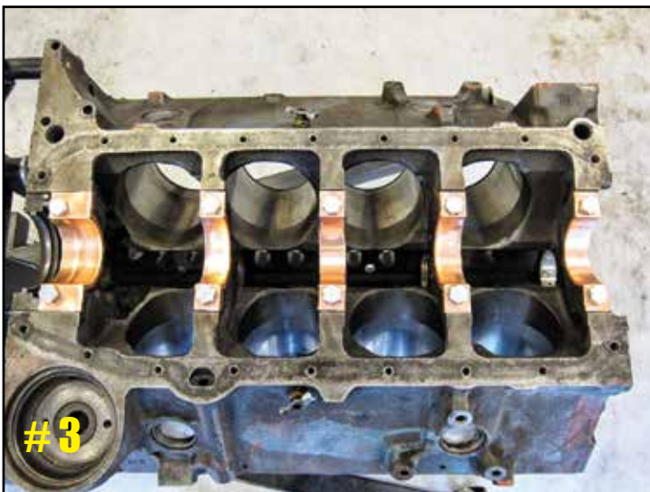
Copper lining of bare main journals to allow 383 crank to be placed in block during clearancing
