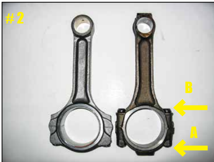
Comparison of stock rod and stroker profile rod
