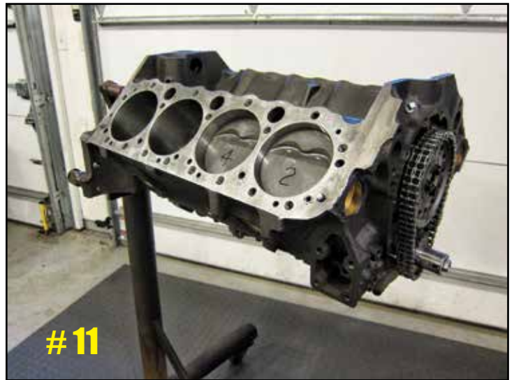
Top view of completed short block
