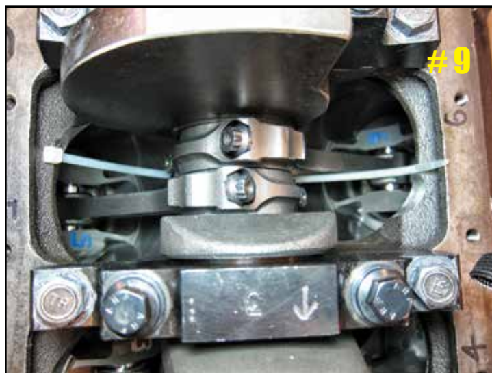
Using a nylon zip tie to check rod-to-cam clearance
