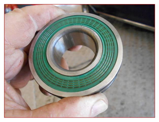
Some bearings have a seal on the other side (permanently sealed) and some do not (lubricated by rear-end oil). If your new bearing has a seal on both sides, this is what the INSIDE seal looks like.
