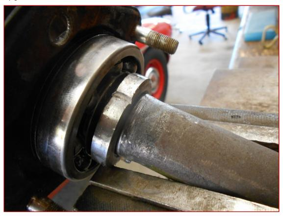
The groove loosens the lock ring enough that it virtually slips right off.
