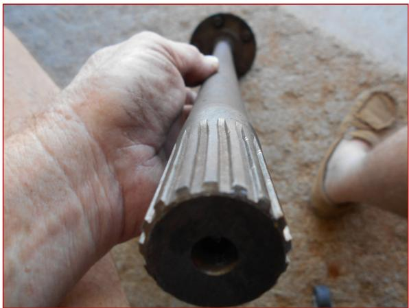
DO NOT, DO NOT, DO NOT FORGET to drop on the bearing retainer BEFORE pressing on the bearing!!!!!
