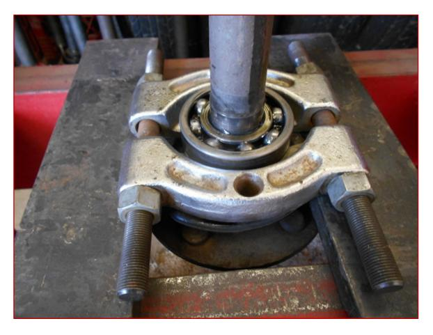
Once the bearing is off, clean and inspect the axle surface where the bearing seats (as well as the rest of the axle).
