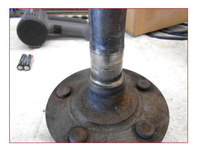
This is the left axle from the 56 Vette. As can be seen from inspection, the splined end has a slight twist (I'm still going to use it).
