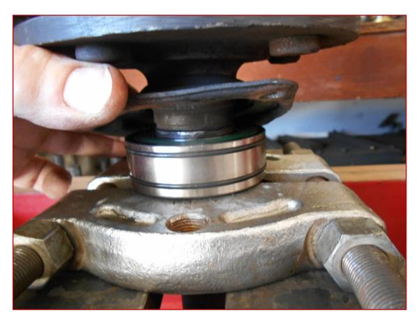
Now press on the lock ring. As mentioned above when pressing on the bearing, I also partially press on the lock ring and then rotate it 2-3 times.
