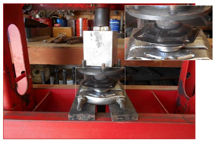
New bearing and lock ring are now pressed on and ready to stab into the axle housing. I also like to use a new gasket.
