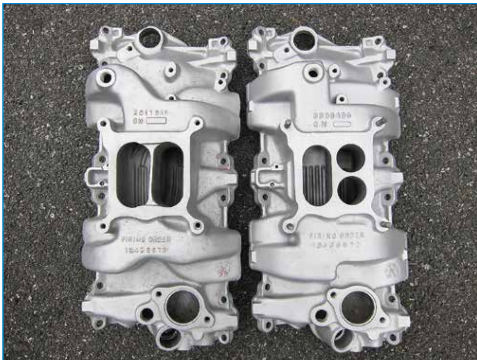
This photo shows the two manifolds side by side, with the Z28 intake on the left and the L79 intake on the right.
