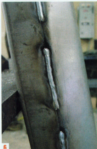
6 Typical welds on the #3 crossmember; MIG-welding is much cleaner than the original A.O. Smith stick-welds.
