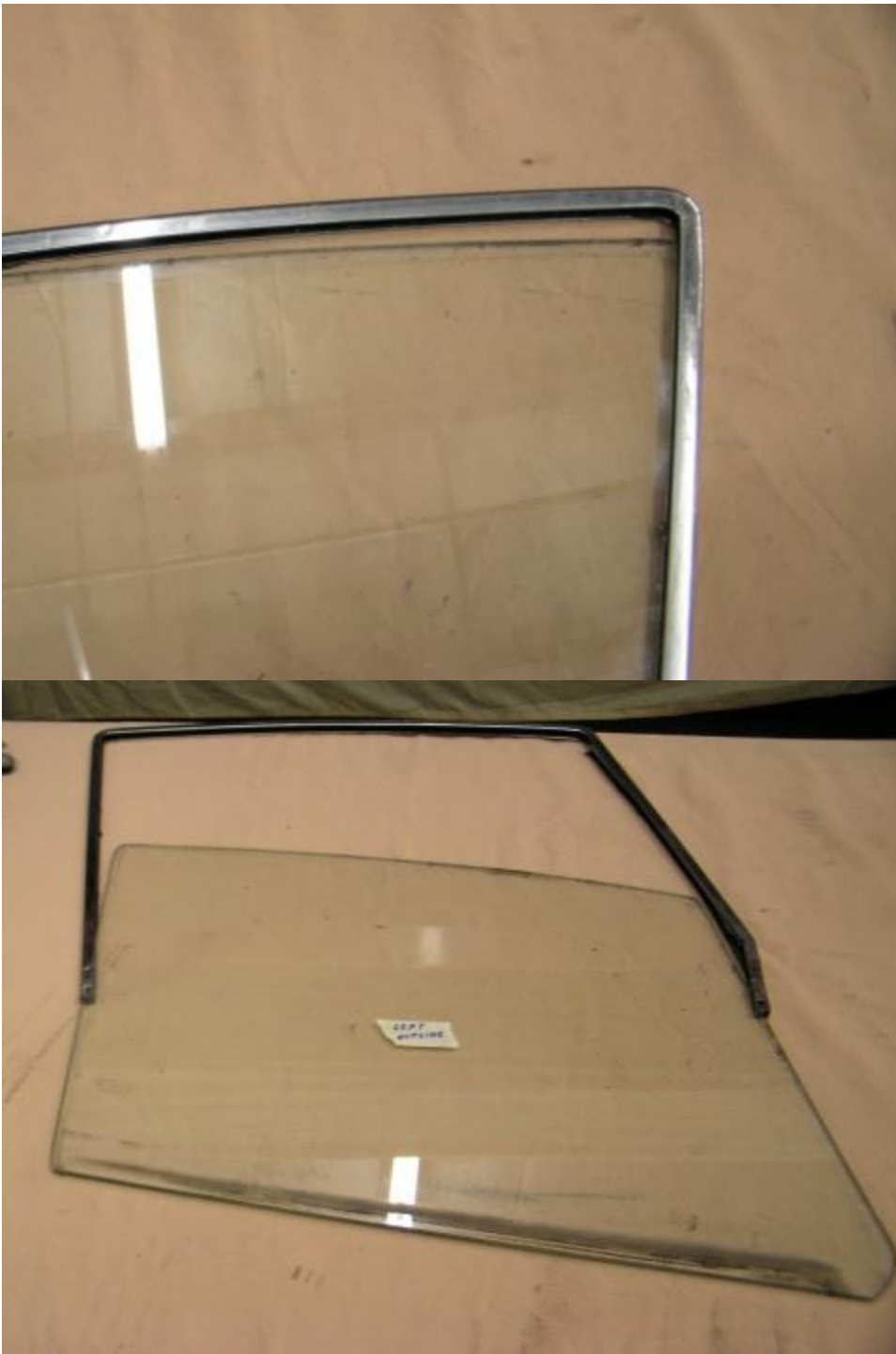
Separate the old seal from the frame. Clean the glass along the edges using a solvent to help remove the old seal residue.
