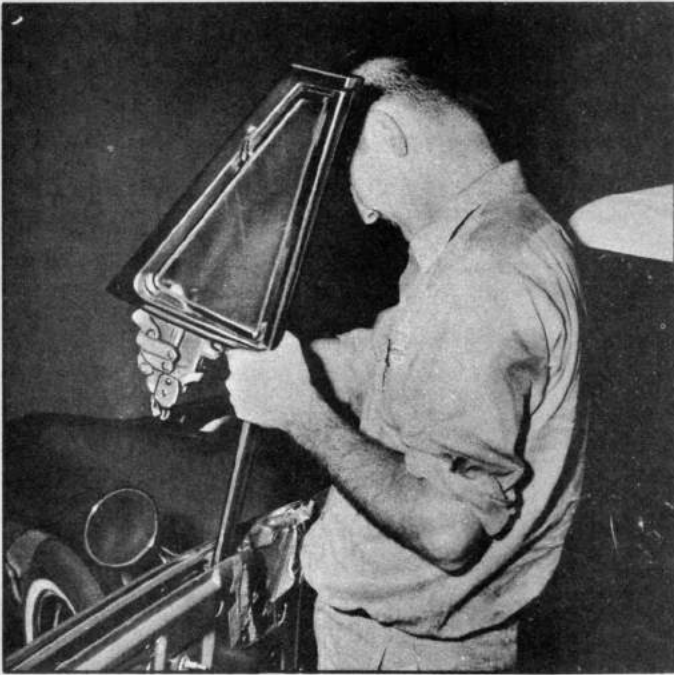
Fig. 40—Removing Ventilator Assembly—867
