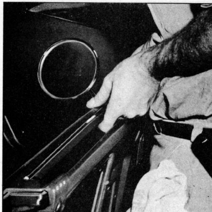
Fig. 45—Installing Outer Seal
