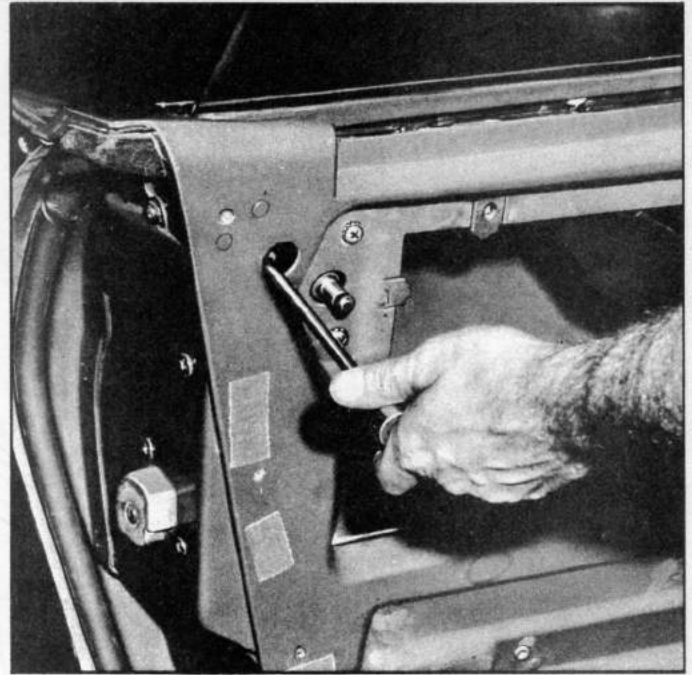
Fig. 42—Removing Sash Retaining Screws
