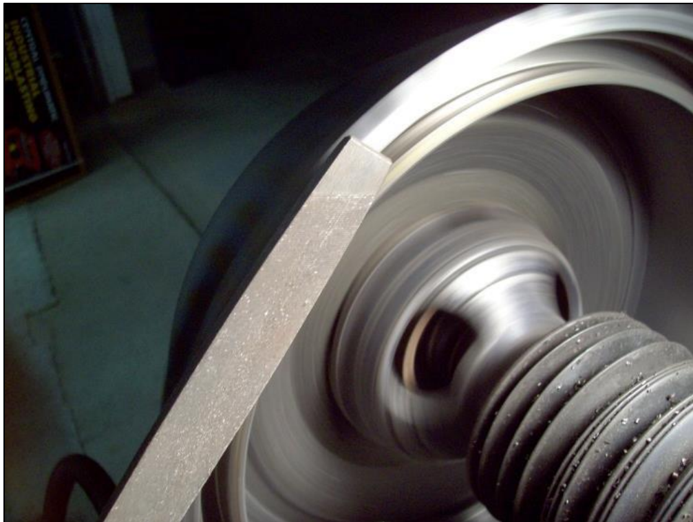
Photo 12: After the flange is completely cut away, I like to use a file to smooth out the cutting lines. I do this while the drum is turning on the lathe ..... BE CAREFUL HERE!!!!
