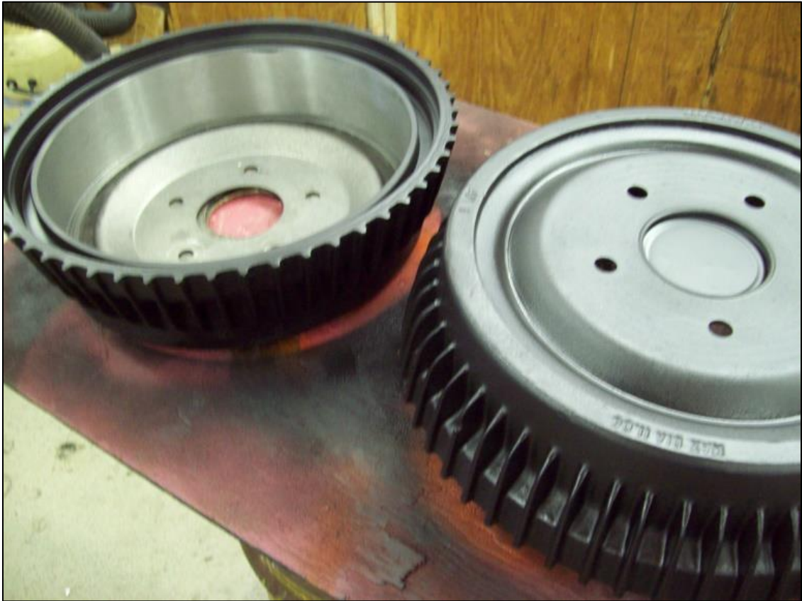
Photo 13: Finished drums after applying a coat of High Heat Black paint.
