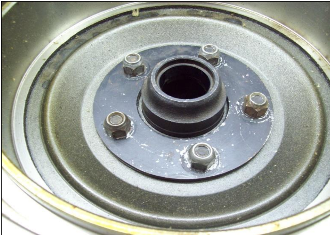
Photo 6: Next, the Olds drum and a regular stock drum are sandwiched between the hub and the spacers and bolted together.
