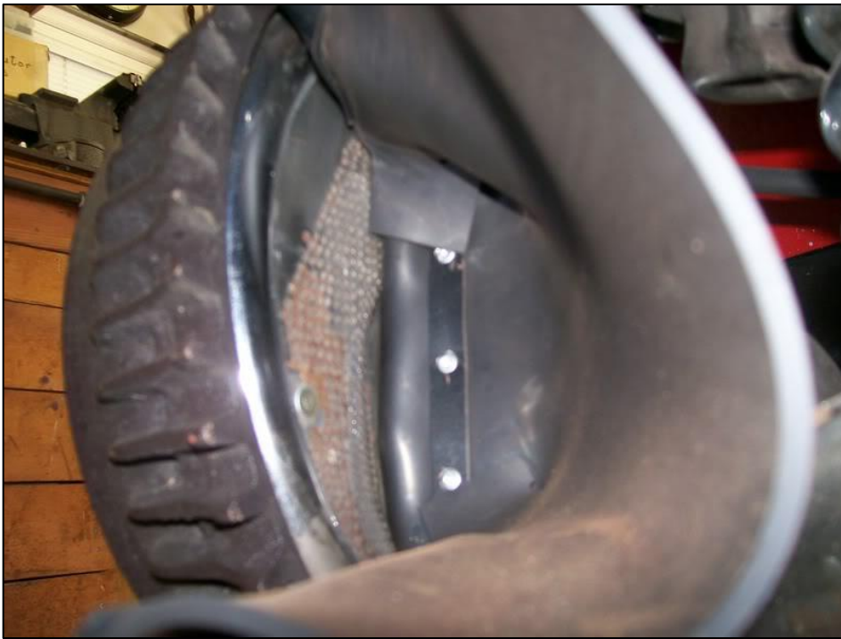
Photo 19: The factory HD brake package included vented backing plates which had irregular cut openings that had wire mesh welded over the openings to keep out debris. Today's prices for HD brake backing plates are astronomical! I borrowed some original backing plates from a friend, traced out the opening pattern on my stock backing plates, marked out a grid, then drilled about 300 holes per backing plate. The forward opening is for intake cooling air and the rear opening is to allow hot air to exit. I also bought a pair of reproduction front air scoops ("elephant ears"), located the proper position on the stock backing plates, drilled and tapped holes (5/16 fine thread) and then attached them with 5/16 in. bolts and used nuts and star lock washers to firmly secure the bolts.
