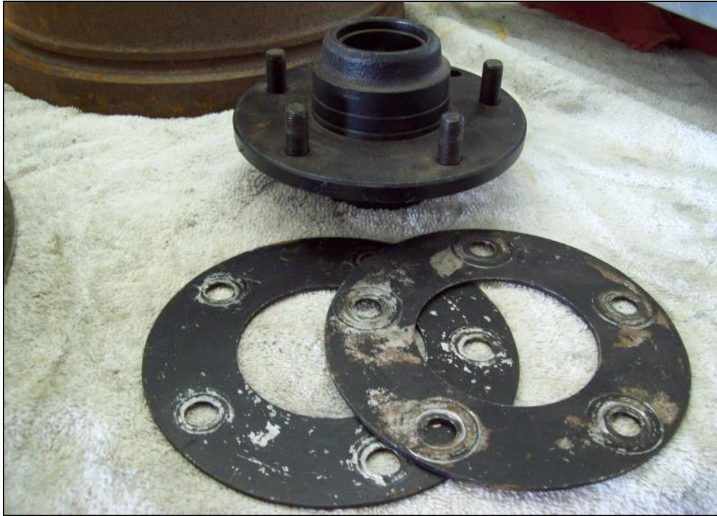
Photo 5: This picture shows the parts that were used to set up the 76-77 drums for pressing the front face inward. An old front hub (from any Chevy or GM car that has the same bolt circle as the Vette, which is 4 ¼ in.). Also, the front faces are cut out from 3-4 old junk drums to make the spacers.
