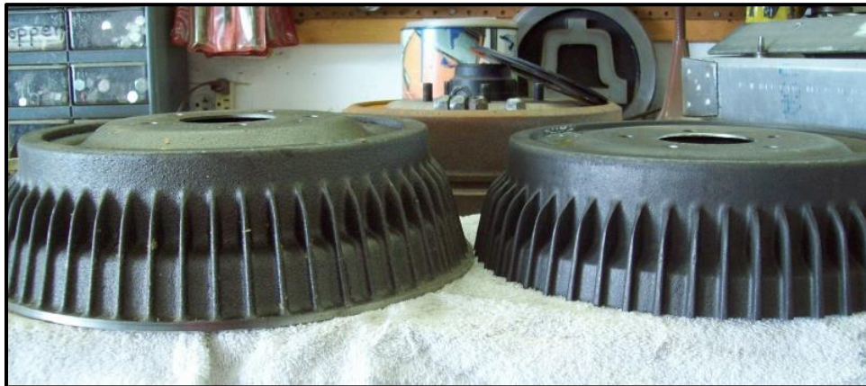
Photo 1: A comparison of the differences in height between the front face of an unmodified drum and a finished drum.
