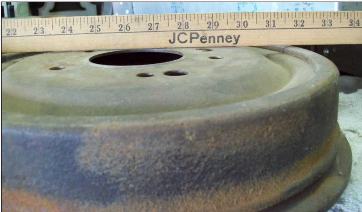
Photo 4: Photo of regular, stock drum simply shows where the plane of the front face is, in relationship to the outer diameter of the drum.
