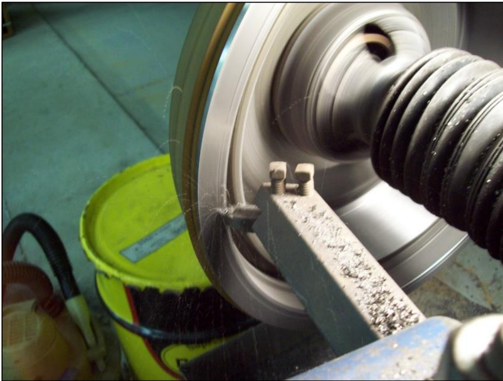
Photo 11: Once the inside corner and braking surface have been turned and trued up, the next process is to cut the outer flange away from the fins to expose the ends of the fins. You better have a few extra cutting blades on hand, because it is possible that 1, 2 or 3 of the blades may get broken once the flange is completely cut away and the cutter begins to contact the ends of the fins. To eliminate, or at least minimize, the possibility of breaking a cutter blade, it is necessary to cut SLOWLY and make VERY SMALL cuts once the fins begin to be exposed
