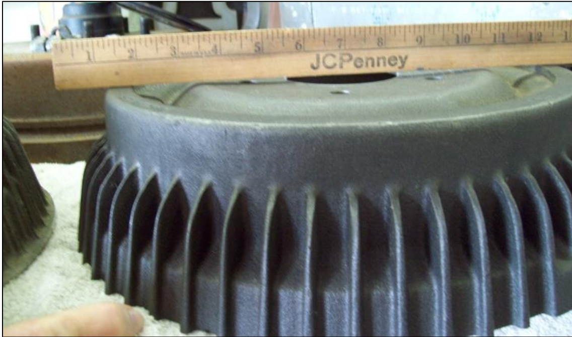
Photo 3: Modified drum... This is the amount that the face of the 76-77 Olds drum has to be pressed inward so that the back of the drum does not make contact with the brake backing plate.
