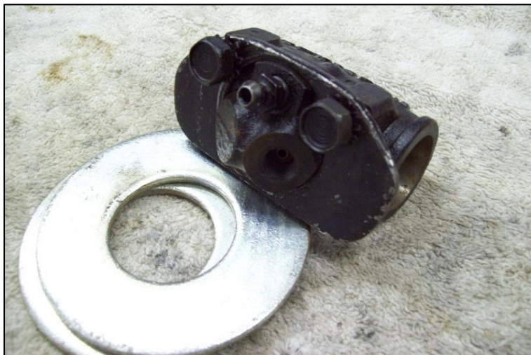
Photo 17: Here are the fabricated spacers for the wheel cylinders.
