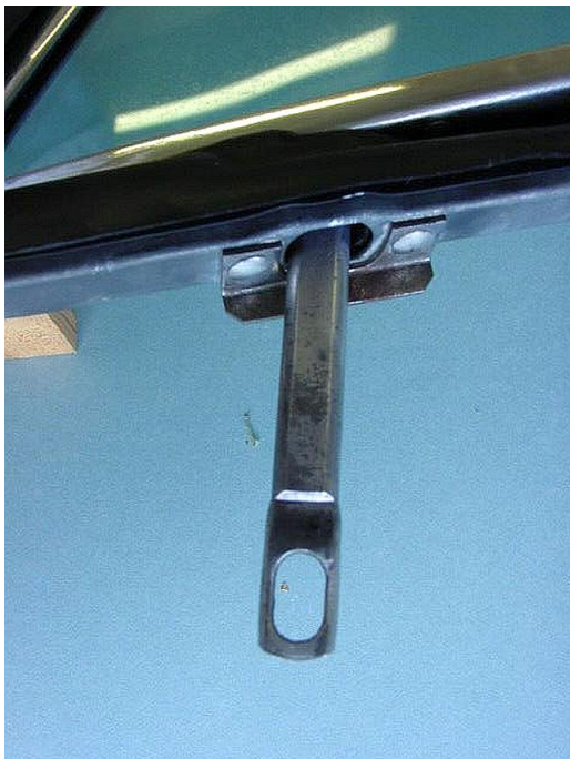
T-Post is riveted to the vent-glass frame.
