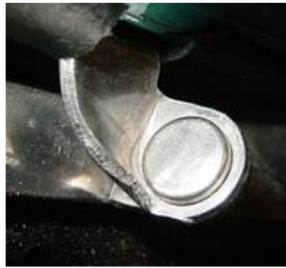
Hinge pivot and rivet on vent-window frame
