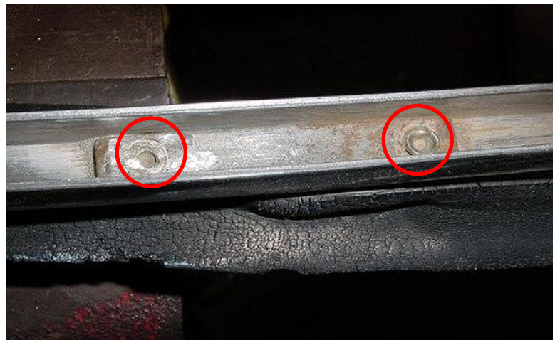
T-Post is riveted to the vent-glass frame.
