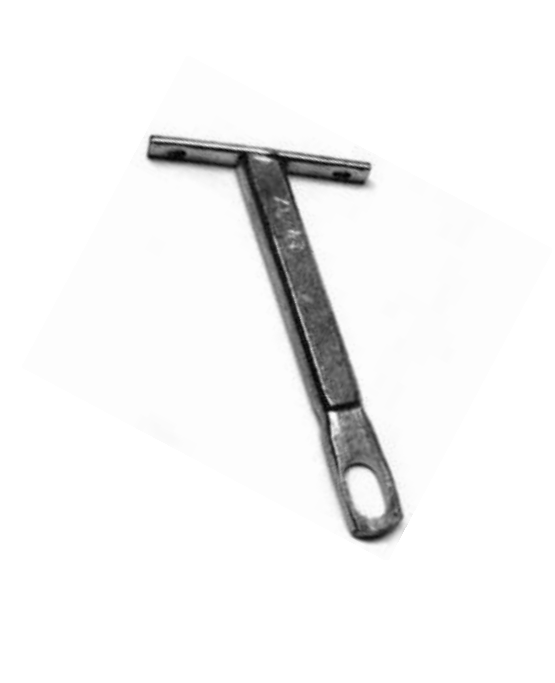
Hinge pivot and rivet on vent-window frame
