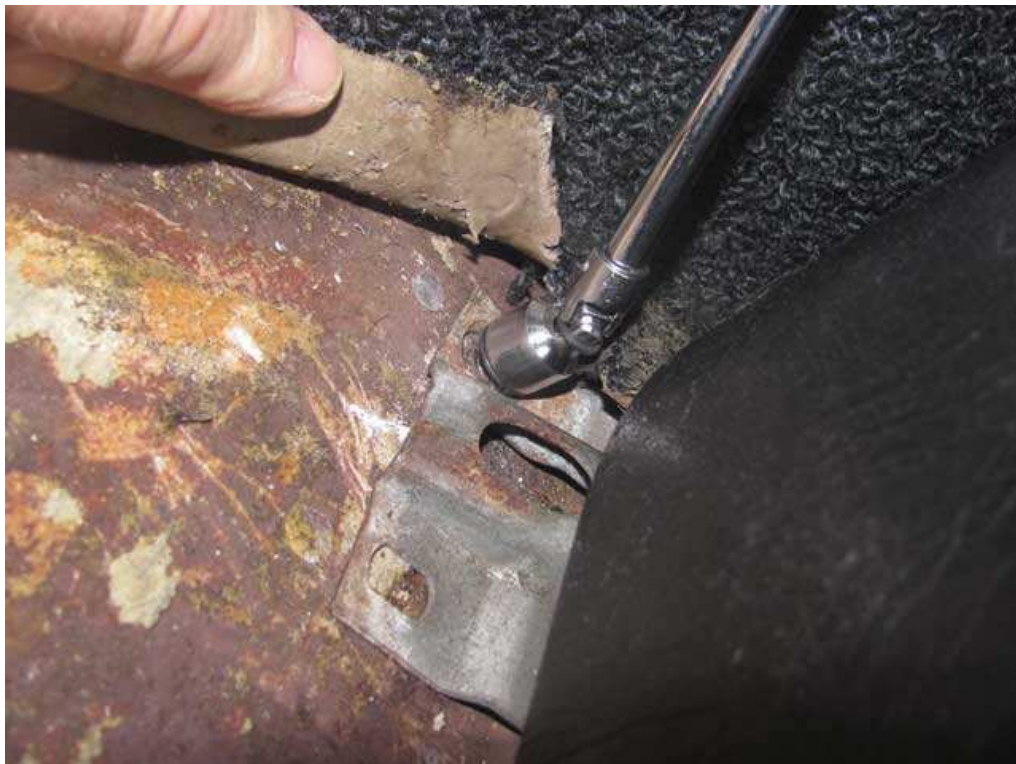
After pushing the seat back, I used a swivel to remove the two front seat track bolts.
