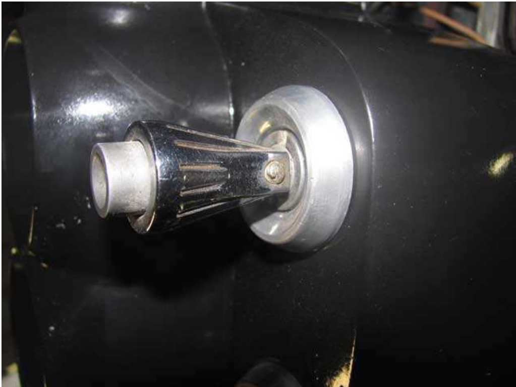
Remove the set screw on the wiper switch.
