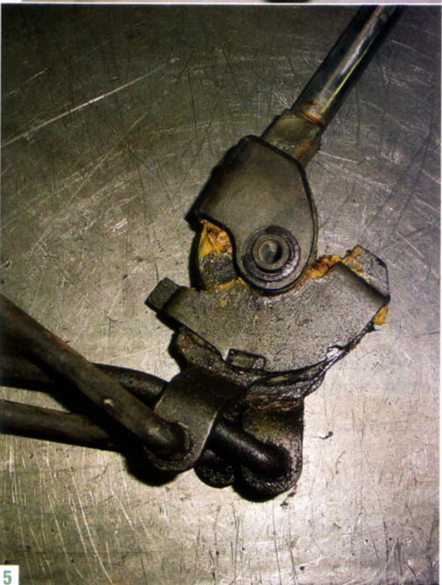
2 The "foot" of the upper lever engages the notch in the lower levers to move them fore-aft.
