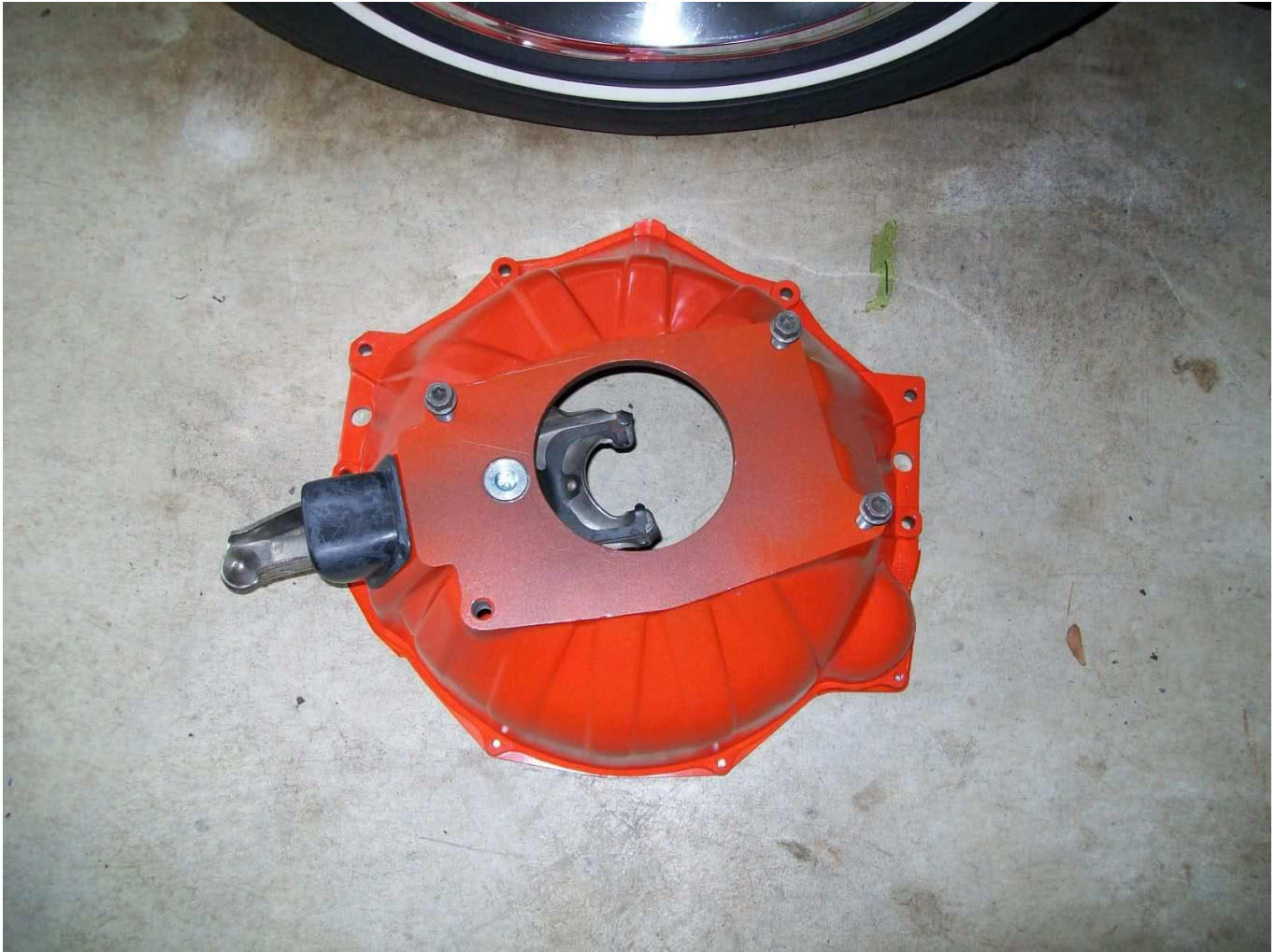
Fig. 4: 1983 Camaro tilted bellhousing (photo by CF member Tom Austin)
