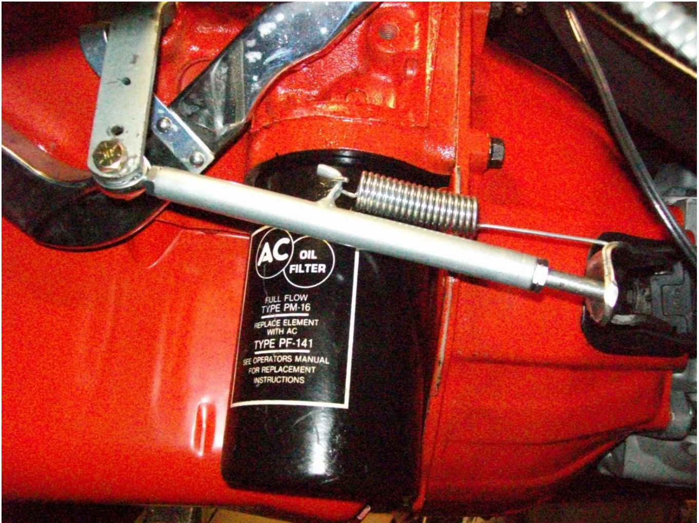
Fig. 5: C2 clutch linkage modification for 1983 Camaro bellhousing (photo by CF member Tom Austin)
