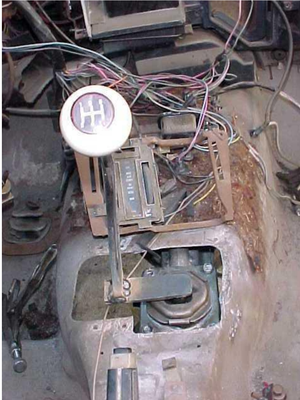
Fig. 7: T5 installed upright (not tilted) in a C3 (photo posted on CF)
