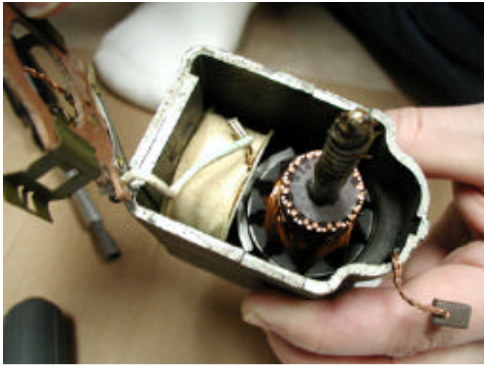
Once the brush assembly is out of the way you can remove the motor for inspection. If it is hesitant to come out DO NOT FORCE IT. Sand the end of the spindle that protrudes from the bottom of the casing (see arrow in next pic)
