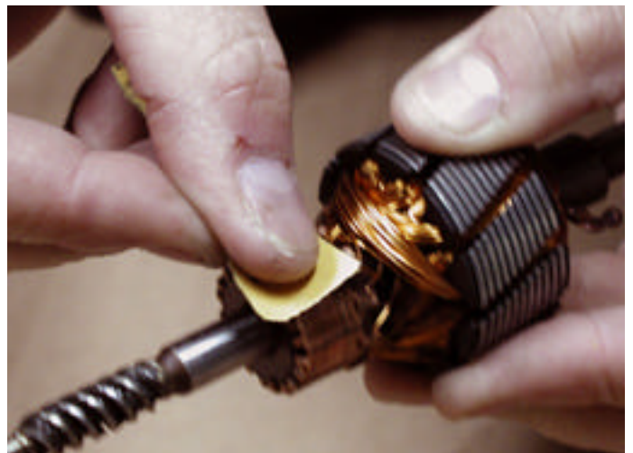
With really fine sand paper (I used 2000 grit) sand away any tarnish or corrosion on the contact area of the motor.
