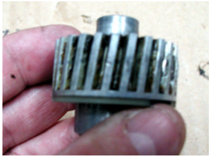
While the opposite side of the same pot metal gear is like brand spanking new. This is because the headlight movement from open to close only utilizes half of the gear's teeth.
