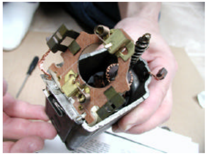
Do not fear the jack in the box brushes, they will spring out of their casing, but will stay attached via copper wire.
