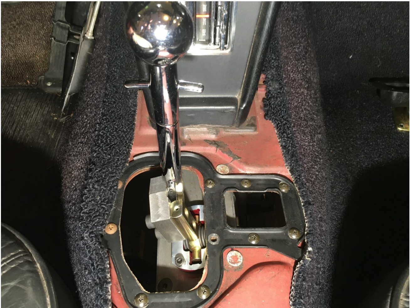
Fig. 7: Modifications to improve T5 shifter location
