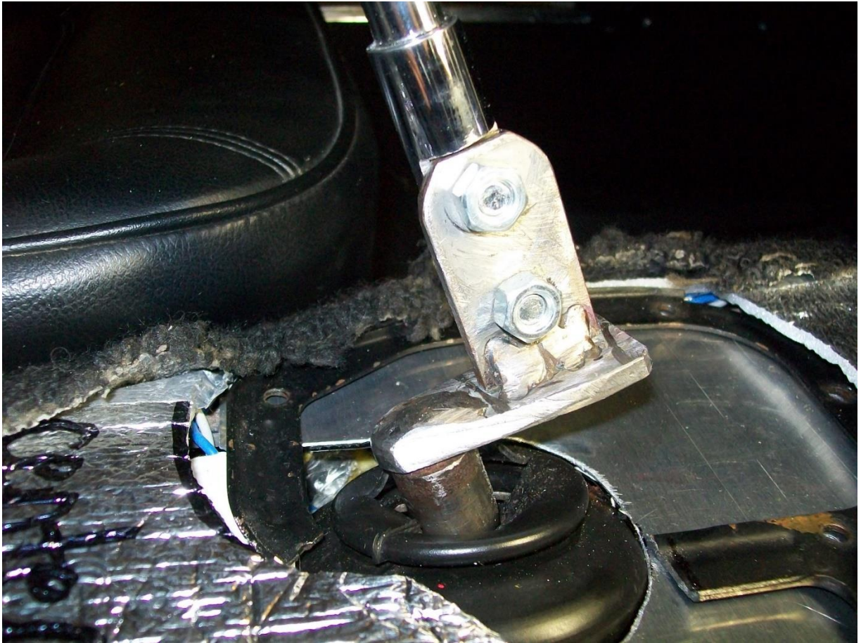
Fig. 6: What's under the console for the T5 in Fig. 1 (photo by Tom Austin)
