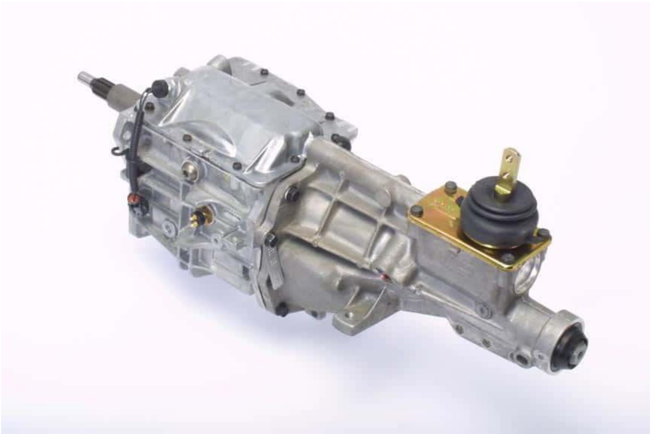
Fig.3: Stock T5 5-speed with shifter centered over the output shaft
