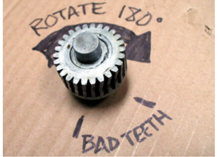
At first I thought I was supposed to "flip" the gear 180° which I soon found was not possible due to its construction. What you have to do, is rotate it in a circular fashion to put the bad teeth away from the worm gear.
