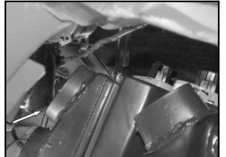
Raingear wiper motor interferred with the vintage air duct.
