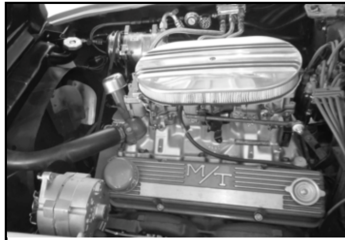
Charging unit, now an alternator, is relocated to the left side. Compressor is located to the right.
