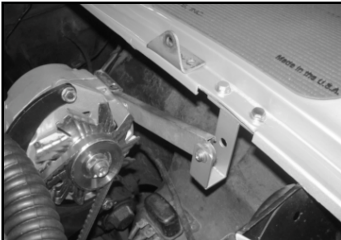
Fabrication is needed to solve hood strut clearance problems.
