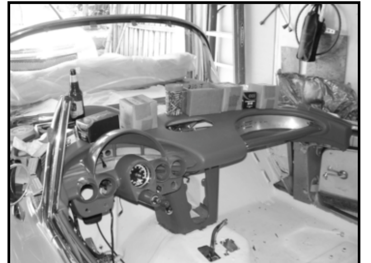
"Project Creep" results in windshield frame being removed for new dash pad.
