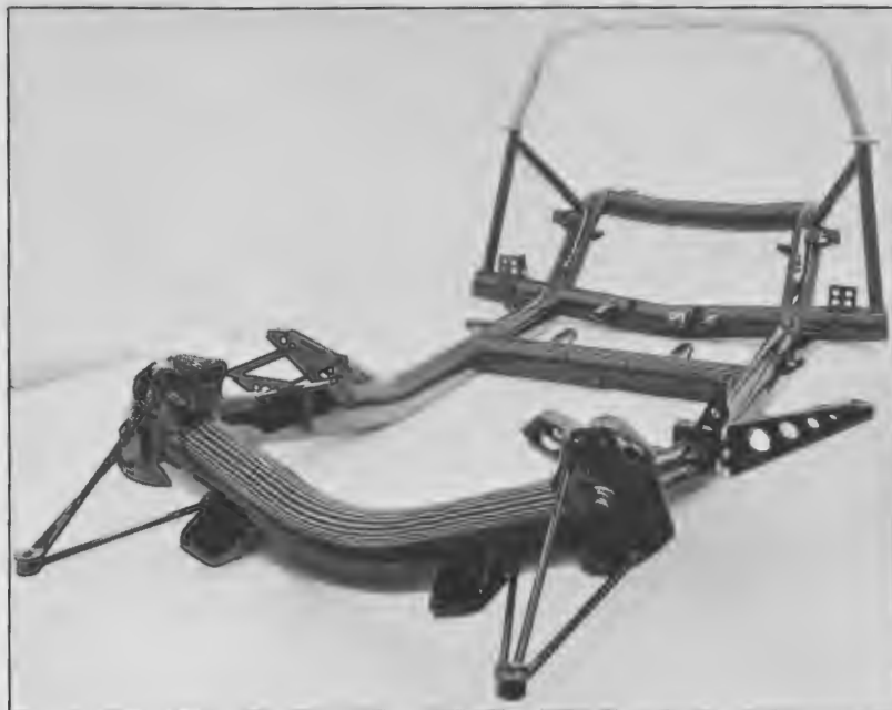
Gradually growing chassis of first Grand Sport is seen from front above and from rear below. Frame's tubular side members ran dead straight in plan view. Transverse leaf spring layout was used, along with standard car's geometry, for rear suspension.
