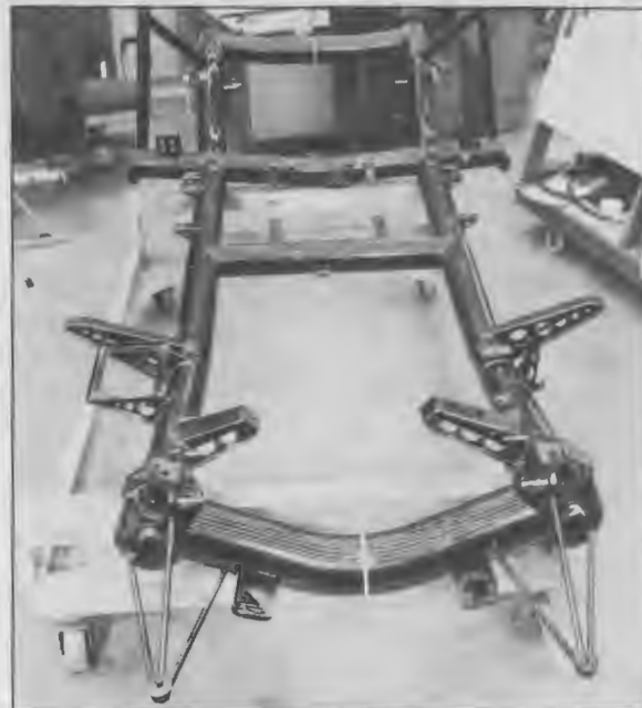
Gradually growing chassis of first Grand Sport is seen from front above and from rear below. Frame's tubular side members ran dead straight in plan view. Transverse leaf spring layout was used, along with standard car's geometry, for rear suspension.
