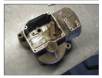
Now for removal of the drive cog from the rear case. Stake both the shaft and the cog (i.e., lightly punch or scratch the cog and shaft to make alignment reference points) to maintain proper alignment on reassembly (A). Drive the shaft from the cog using a drift. Remove the shaft and link assembly (B). The rear cover (C) can now be cleaned and prepared for plating along with the front cover.
