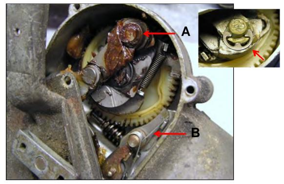
Now remove the cover and linkage assembly/shaft from the motor housing. Inside you will get a better view of the gear mechanism and the various links and levers to control the run and park functions. Clean excess grease from the area.
