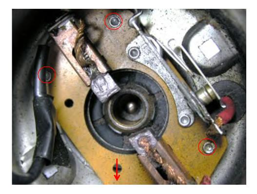
After disassembly, organize and clean the parts for a thorough restoration. The 3 main parts for plating are the motor case, front cover, and rear cover. The main housing can also be cleaned. All other small parts may require light cleaning and detailing.
