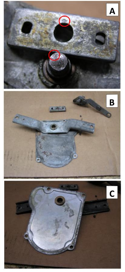
The end case cannot be plated unless the brush board is removed. If desired, simply drill out the 4 small rivets from the inside and lift the board out.
