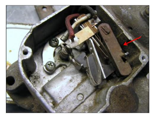
Desolder the red and black wires from the switch. Pay careful attention to protect the wirewound resistor from heat and physical damage.
