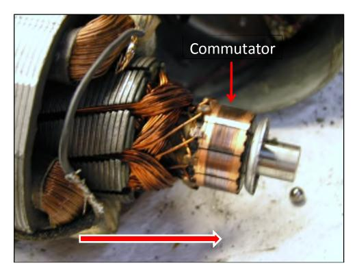
This one needs new brushes and a new brown lead wire. Note one brush was installed backwards previously. This unit was worked on in the past. The thermal breaker (box) can also be seen below.
