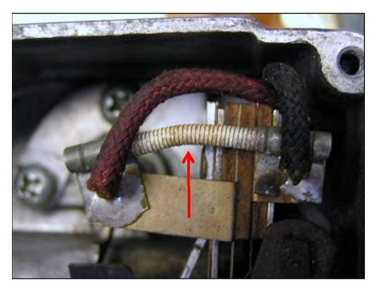
Remove the 2 screws securing the switch. Carefully slide the switch out of the housing, around the park trip lever (arrow) and out towards the left.
