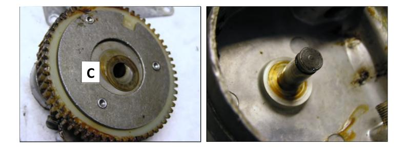
Now you can remove the armature from the housing from the commutator end (where the brushes make contact). There will be a bearing ball, felt donut, and spacer/disc located in the motor case bearing. Sometimes the ball will be stuck to the end of the armature.
