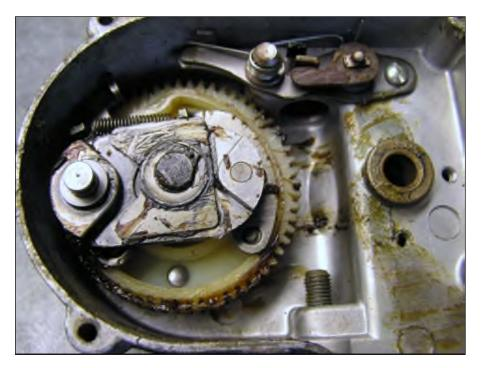
Remove the C-clip (**A**) and shim washers (**B**) from the shaft, and lift the gear out of the housing. Note there will also be a shim washer (**C**) below the gear.
