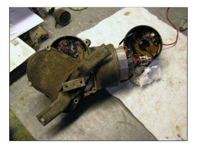
Remove the top cover from the housing by removing the 4 screws and the cable actuator attaching hardware. There will be different actuators if the car is equipped with windshield washers or not. Inside you will see the main switch and the park trip lever. The lever to the right is the cable actuator lever which is controlled by the dash knob/cable.
