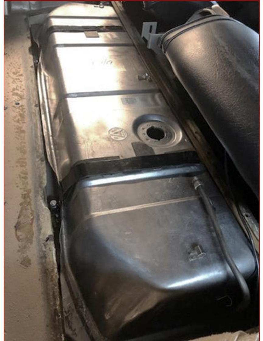
14) New tank in...Did everything but stand on it..... Strap forward terminations are important. Double check your under-car front tank strap channels. That is where the, just behind the seat, strap terminations are. When inserting the tank make certain the front ends of the straps stay where they are supposed to. Otherwise plan on spending some extra time under the car re-positioning them while the tank is wedged in. Don't ask me how I know>>>>>>>>
