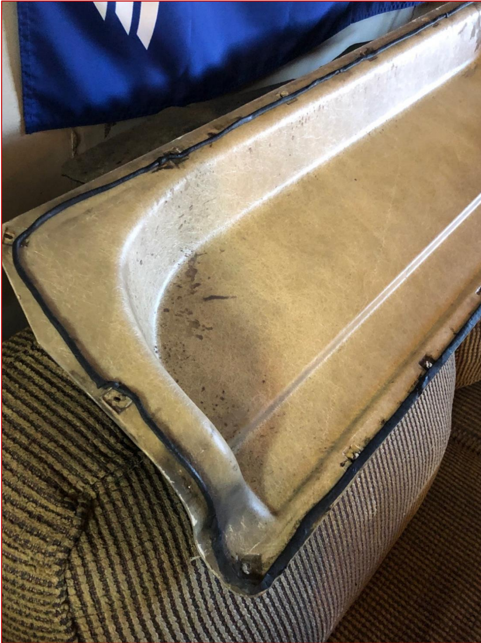
13) Prep tank cover with 3M sealing strips (Dum Dum). Just waiting for a little help to simply lay the new tank in its place..... Yeah right! Crowbar is ready!!!!
