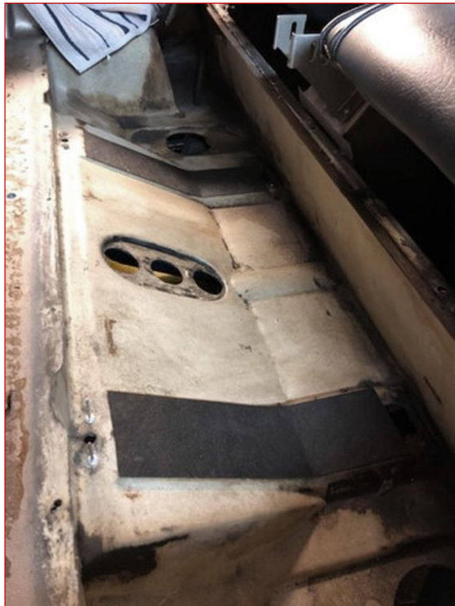
8) While I'm waiting for parts I glued in the anti-squeak pads....I sure don't want the pads wondering around while I'm muscling the new Tank into place.....
