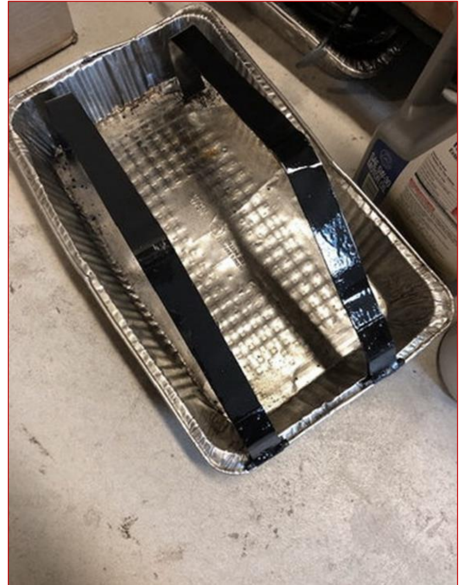
10) Using the original tank straps, reshaped and painted left the bent areas alone!!! Also checked the Strap grab plates under the tank compartment....Making certain they were not rusted away....All good!
