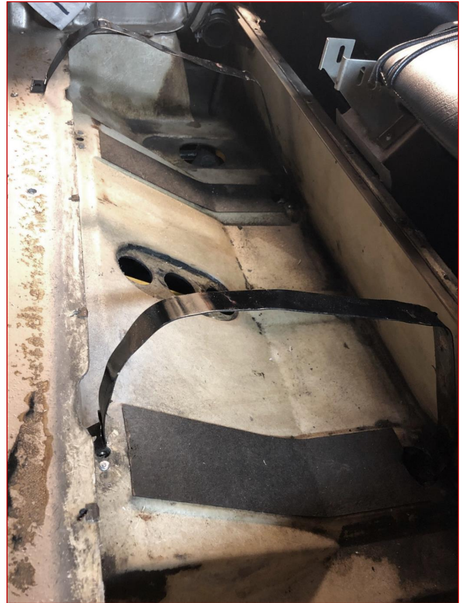
12) Tank Straps ready...Hope I have enough hands. Refasten all the screw nuts that were actually in pretty good shape.
