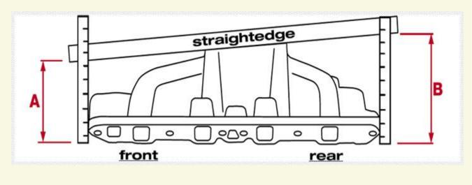
Measured carb height "CH" for GM aluminum intakes:
