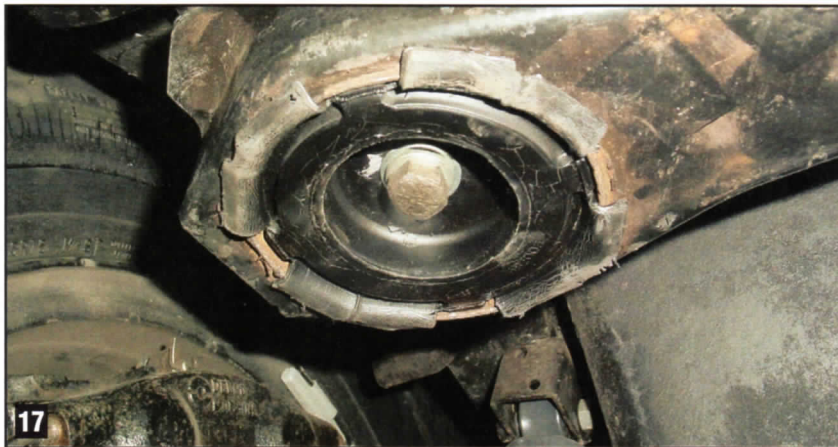
17 The crossmember and new bushings back in place, through-bolts torqued, ready for another 40 years and 90,000 miles.
