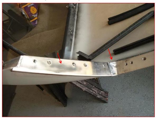
Then you can attach the **WS** for the top and backside of the window. The little piece that of **WS** that is between there and the back trim can be installed now or wait until the other back **WS** is in place. If you wait it will allow you to fit everything nicely.
