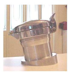
The two units required different designs due to the tank configuration being different (I suspect his was not the original tank). My goal in each case was to make the cap functional, integral to the tank (yet independent of the body) and cosmetically aligned to the body.
