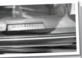
ABOVE: Distinguished by the "9" in the eighth digit of the VIN, this 1978 Pace Car proves to be legit. Regular production 1978 Corvettes ran from 400001 through 440274 or 40,274 Corvettes. Pace Car production added an additional 6,502 units and numbered 900001 through 906502. (Photo: Bob Stevens Archives)
