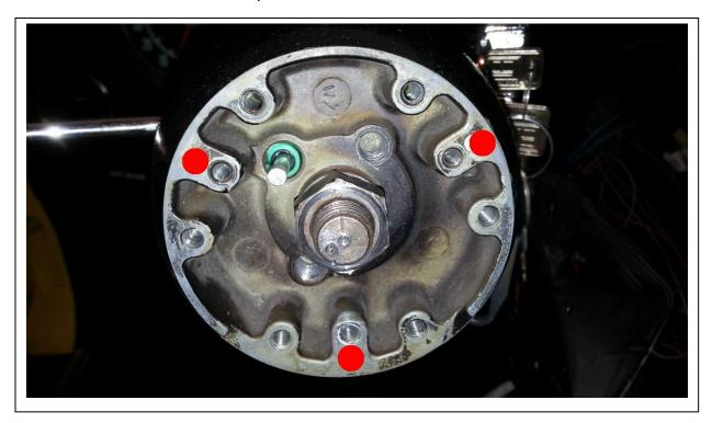
Install the bolt and washer as shown.
