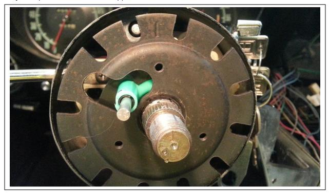
Install the *shaft lock cover* and the three screws that hold them together. Please note that the *shaft lock plate* has grooves and can only be installed in one position. A *locking plate clip* is then installed – mine was missing so I didn't show it here, but in the above photo you can see a groove in the column where it slips.
