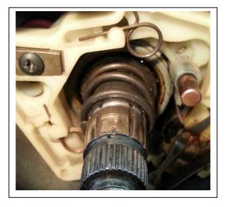
The horn contact, which is the button on the right of this photo, when grounded to the shaft, should sound the horn. Use a piece of wire or even a screwdriver to test this. If it doesn't sound, you have another problem besides the parts in the upper steering column.
