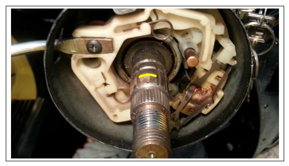
Install the *shaft spring* onto the *steering shaft*.
