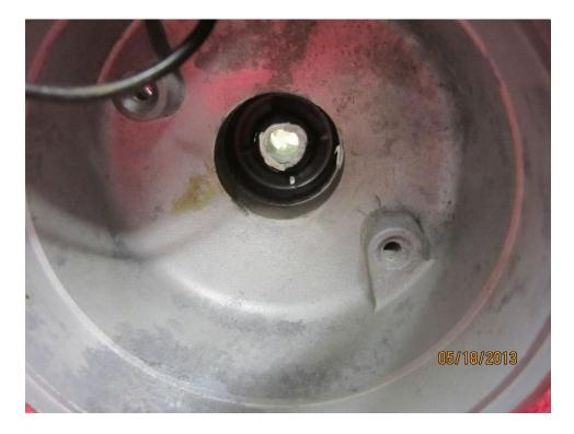
Feed the two wires out of the hole and keep pulling them through as you slide the armature into place.
