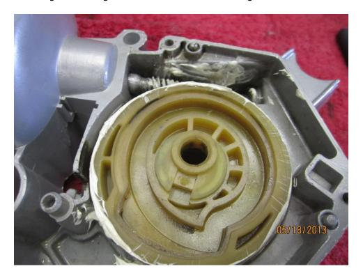
Run the motor for a minute and bring in the adjuster screw until it light loads the worm, you'll actually hear the motor smooth out, if you run it in too far it will slow again. Tighten the lock nut
