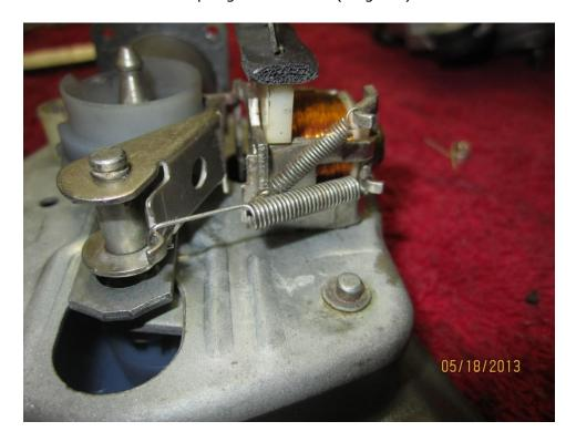
An E-Clip holds the ratchet arm on and a spring holds the plastic gear in place
