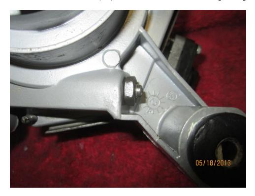
The center shaft is in three pieces, the shaft, follower cam and stop cam. They stack together with the shoulder on the stop-cam locating the follower cam into the arm on the shaft
