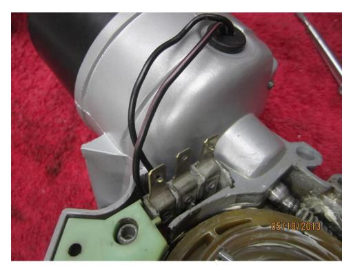
A 20 ohm resistor seems to be the correct resistance, but a 5 watt 22 ohm resistor works to replace the missing or damaged wire resistor.
