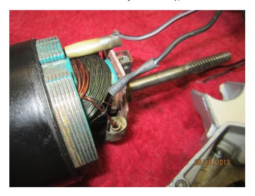
Grease the inside bearing where the worn shaft goes through with a light grease (white grease works well)
