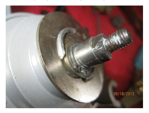
Mine also had a thin steel washer between the spacer and the plate, no mention of this in the manuals.
