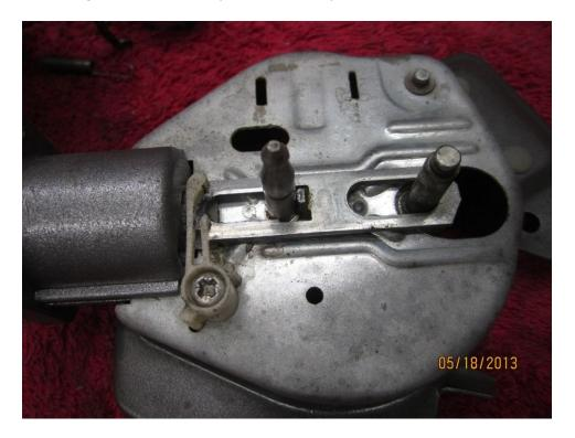
There are two little alignment pins on either side of the screw to locate it correctly.
