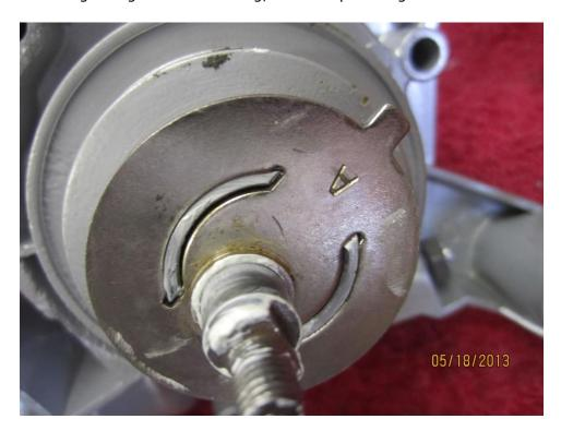
The plate had a shoulder sticking out around the shaft hole, that goes to the outside (away from the housing)
