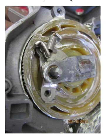
Make sure the three parts are stacked and sitting down together properly (the middle lever has the large hole that must be centered on the pin from the bottom one)
