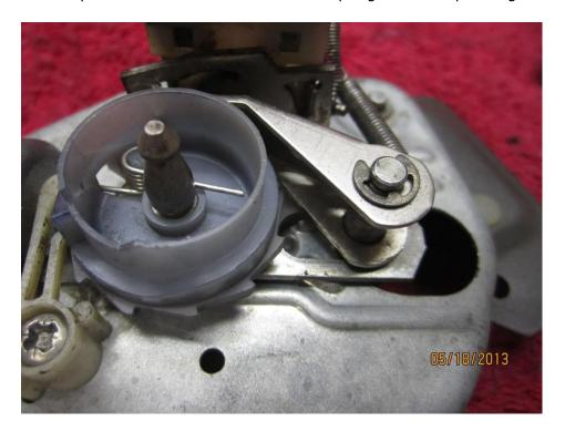
With the motor in the parked position, turn the cam wheel so the pin on the motor locates in the curved slot (greased in this picture) and put the two parts together and bolt everything up.
