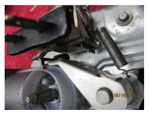
The orientation of the spring for that arm (diagonal) holds it down on the cam track of the gear
