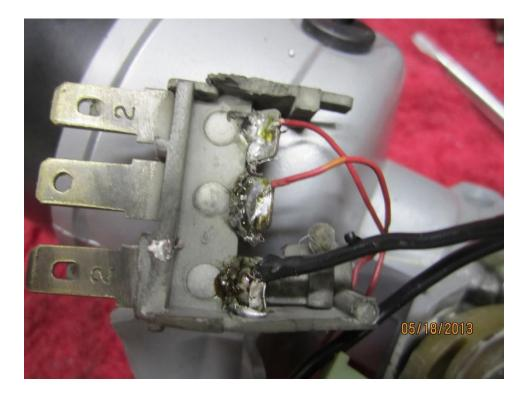
The small red wires both go over to the stop relay and attach to the electro-magnet.
