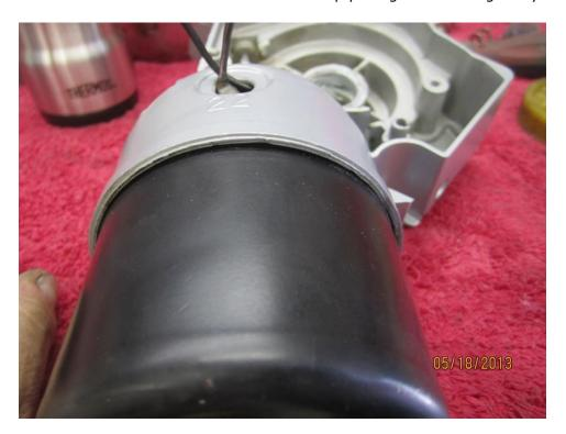
Careful not to pinch the wires. Align the two long screws and lightly snug them
