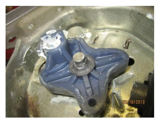
Put the electromagnet in and use a large screwdriver to spread the tangs locking it firmly in
