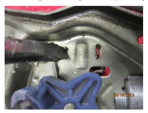
The ratchet arm can go on, notice in the background the arm for the electromagnet arm riding on the plastic gear
