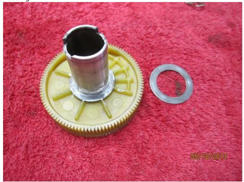
Grease in inside of the bushings and put some extra in the cavity between them
