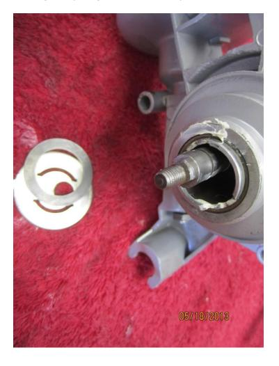
Washer goes against the housing, then the plate aligns with the two arcs
