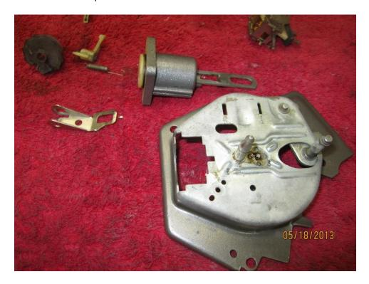
Shove the piston in with your thumb and slip the pump into the housing. The pump body has two slots that line up with the housing
