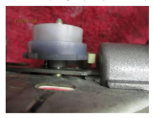
Flip it over and drop the cam wheel onto the shaft and install the locking washer. I use a small socket to press it into place
