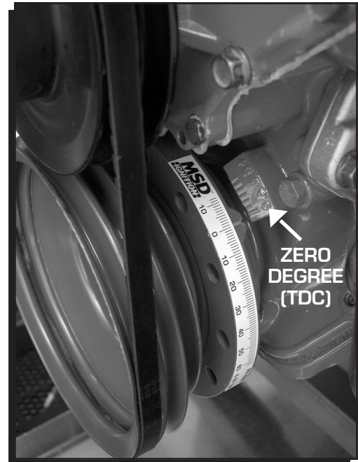
Figure 9 The Timing Tape Installed.
