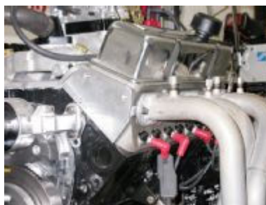
Each combination received a set of aluminum Pro Comp cylinder heads. Each head features a
