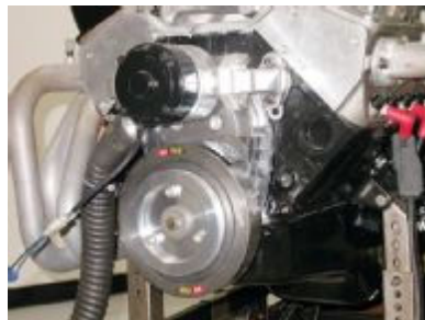
The motors were run on the engine dyno with a Meziere electric water pump and a Pro Street
