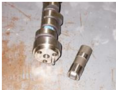
Wanting impressive street performance, both 400s were equipped with hydraulic roller cams.
