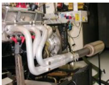
Both motors were run on the engine dyno with the same set of 1 3/4-inch Hooker headers.
