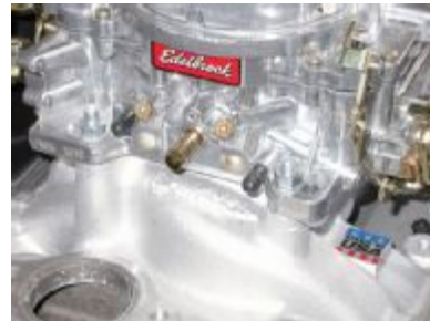
Both 400-inch small-blocks were equipped with Edelbrock carbs and Air Gap manifolds, but e
