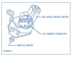
Do not jump the ISC motor after the plunger reaches the fully-extended or retracted position
