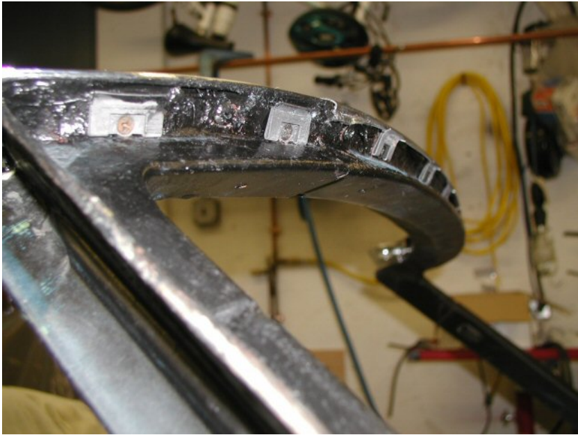
Reveal Molding Clips In Place
