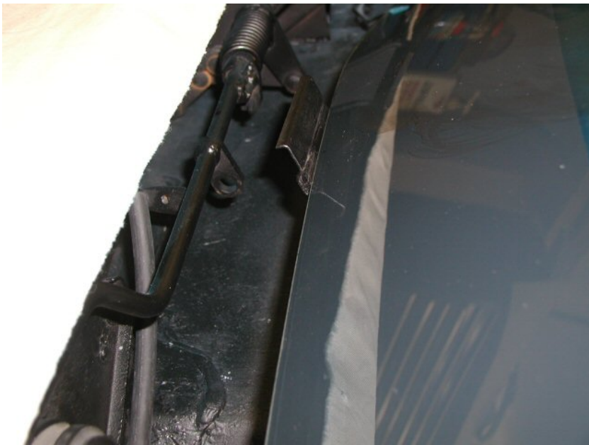
Windshield Bottom Rest (and wiper park stop)
