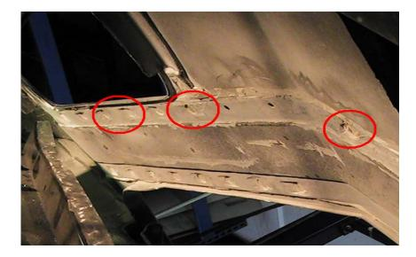
Once you have the rivets all removed, it is time to bond in the new upper header. This time we are not using rivets to hold the header, we will be bonding using SEM 39747 panel adhesive. 3947 adhesive will bond fiberglass to metal, metal to metal and just about anything else you want to glue. It does take a special gun to shoot this mixture, but it is well worth the expense if you are going to do more than one. I'm not so sure how well it would work out for a one time application cost wise.
