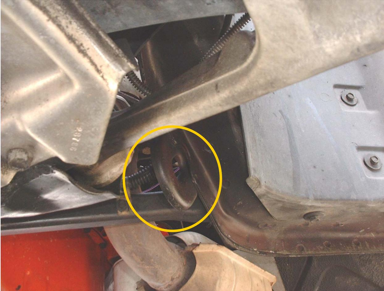
This is a front tow hook. It is so very important that when your Corvette requires towing you use these hooks. If the operator does not use the hooks and attaches the retaining chains to a suspension arm, something will be damaged.
