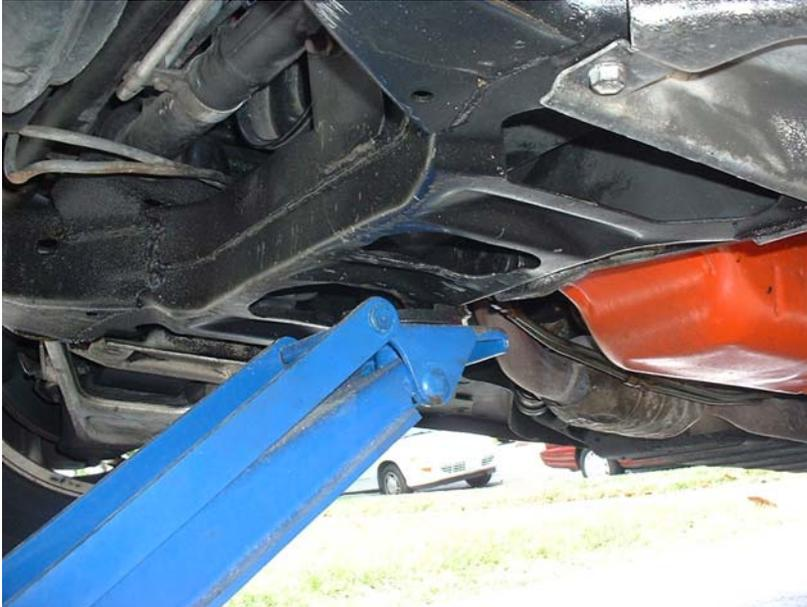
One option for lifting the front, is to have a jack that reaches and lift from the front cross member.
