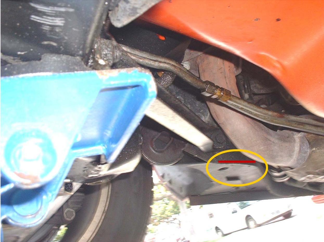
To use jack stands, in the front, use this area to place the stand. This is a seam in the frame rail that is more than strong enough to support the weight of the vehicle. **Note the red line!** That's where the stands should be placed. This is a good place to put a lift arm, too.
