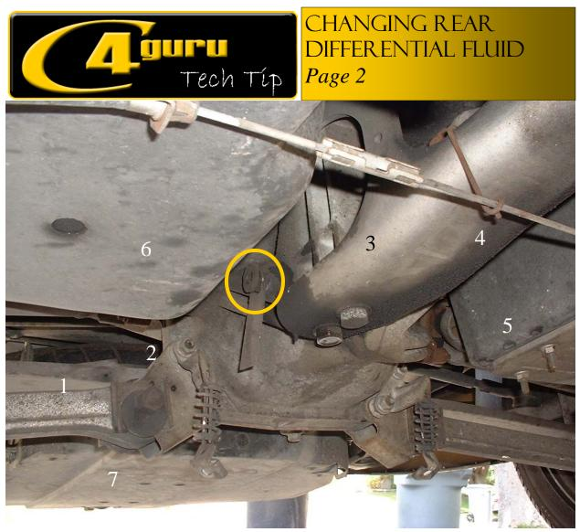
This is the rear differential of a 1992 Corvette with an automatic transmission. All years look the same, regardless of the transmission.
