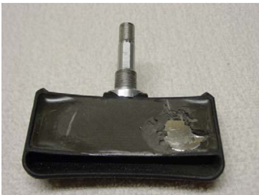
Battery Exposed (Negative Side)
