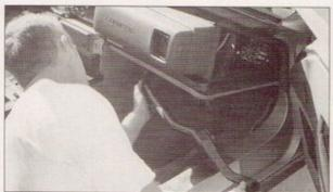
We had the most fun (yes, I'm being sarcastic) pulling out the ductwork for the floor vents. If your Vette is equipped with an aftermarket stereo, we suggest that you take the time to remove it — otherwise, you'll rip out wires when the duct is removed.
