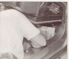
The side window defroster duct can now be disconnected, which leaves us room to remove the ECM. The manual, of course, doesn't say how, it just says "remove ECM."
