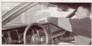
To remove the dashpad, grab it at the defroster vent and pull back. If you love your Corvette, this is going to be a really hard step for you because it'll feel like the dashpad is going to break before it snaps free. The manual didn't tell us how to remove the pad, but thankfully we figured it out before we destroyed it by trying to pull it up.
