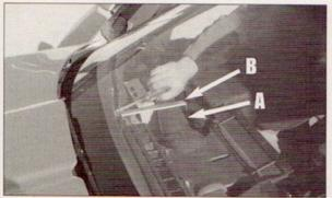
The next item slated for removal was the AC duct (arrow "A"). However, the manual forgets to mention this brace (arrow "B"), which is in the way.
