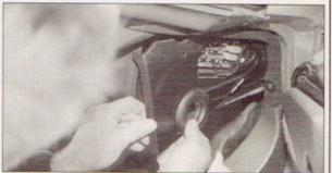
Moving to the possenger side, we found that the carpeted panel cannot be removed the same way the driver's side was, so we needed to gain access from the top. We began by removing the trim panel for the fuse box. Right about now, we're thinking that we should abandon this project — but hey, we're troopers, right?
