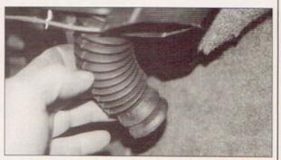
With the lower portion of the dash removed, we now have easy access to remove the driver's side defroster ducts. The manual told us that we needed to remove this piece, but didn't tell us exactly where it was, or what it looked like.
