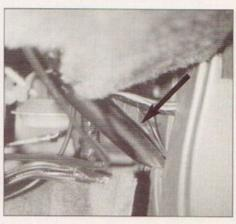
Trying to remove this brace, which goes from the passenger side door pillar to the inner dash structure, almost stopped us in our tracks. It was next to impossible to get a wrench on one of the bolts, and when we got there, it was on so tight, we thought it had been welded on!
