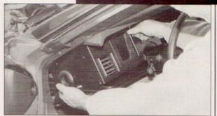
The instrument cluster is the first item to come out. Be sure the tilt lever is removed first.
