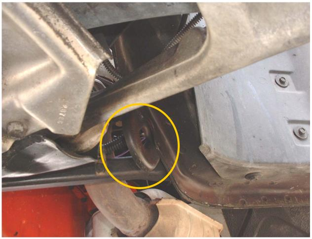
This is a front tow hook. It is so very important that when your Corvette requires towing you use these hooks. If the operator does not use the hooks and attaches the retaining chains to a suspension arm, something will be damaged.
