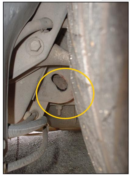
Please note this hook - that's the rear tow hook. It is located forward of the rear suspension. This picture is taken from the FRONT of the rear tire, between the tire and the wheel arch. I suggest painting the rear hooks, too. They are hard to see... so bright red would help a lot.
