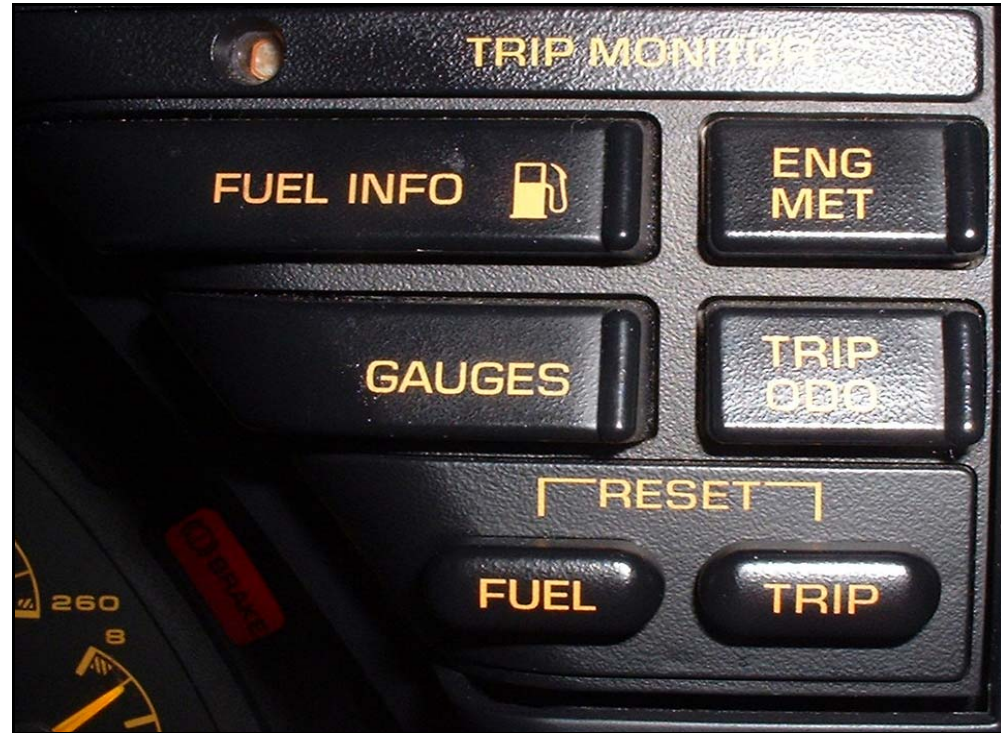
Photo 4 - The Trip Monitor, above, is used to navigate through the various functions of the CCM, detailed instructions are on Page 4 . This photo is of a 1992 Trip Monitor; 1993 is identical.
