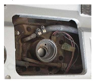
**4.** There is a single three wire harness that services the fuel pump and sending unit. There is a small, white plastic clip that must be removed prior to pulling the connectors apart. Compress it with a pair of needle nose pliers and remove it. Now
