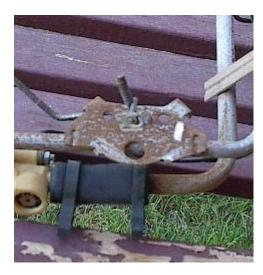
**8.** Now that it's apart, use some 600 grit sandpaper and gently sand the CONTACT. DO NOT sand the windings or you will ruin them. The contact is mounted on a thin piece of springy metal, so use a finger behind it to support it as you sand. Sand it until it has a shiny, new surface. Next, soak a Q-Tip in WD-40 and GENTLY clean the
