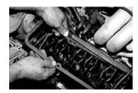
**14:** Put the new valve cover gaskets into place. The side of the gasket with the double holes goes to the top of the head.
