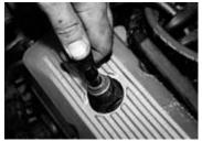
**18:** Install the air inlet tube into the passenger side grommet and the PCV valve and hose in the driver's side grommet. Screw the oil filler cap onto the passenger side valve cover.
