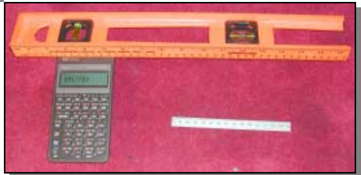
Figure #5: The components of an inexpensive camber gauge.
