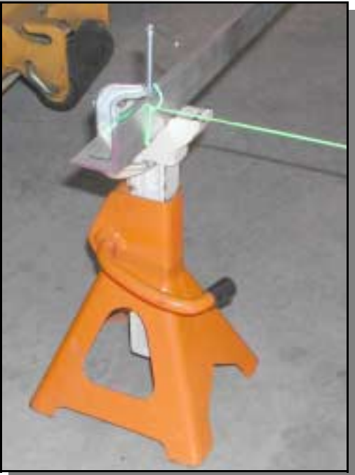
Figure #11: Jack stands hold the cross pieces.
