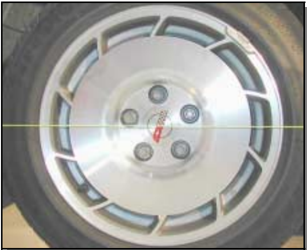
Figure #12: Center the strings vertically on the wheels.
