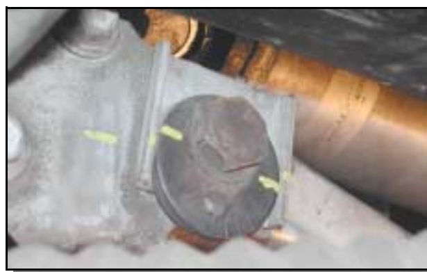
Figure #9: Cam bolt marks help gauge adjustments.
