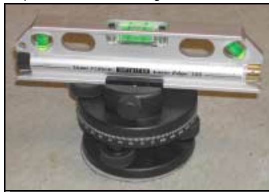
Figure #2: A laser level is one way to set up your leveling pads.
