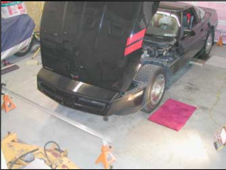
Figure #10: Parallel strings can be used to measure toe.
