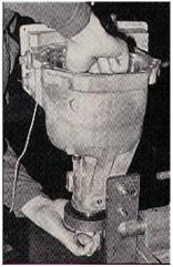
10. Install the direct thrust washer, installing the locking tabs into the direct apply piston. Install the thrust bearing, then the thrust washer plate which si identified from the rest of the direct plates by the tooth missing from the outer edge and a notch on a tooth on the circular ground side of the washer. This side goes down on the thrust bearing.
