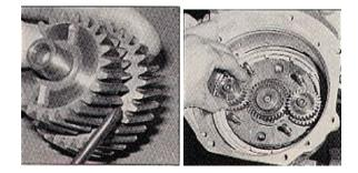
14. Install and time the pinion gears. Each gear bears a timing mark. Install the first two pinion gears opposite each other and with the mark to the center. The next two pinion gears are installed with their
