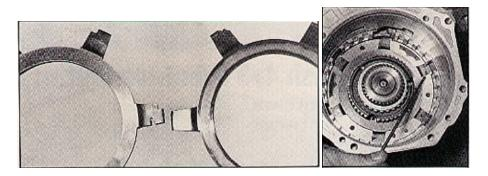
3. The old-style direct thrust washer (above right) was replaced in mid '85-early '86 with the revised washer on the left. Note the special locking tabs on the fingers that keep the washer secured to the direct piston. The problem with the old-style washer was that it would rotate from side to side and notch into the side of the case and prevent the piston from applying or releasing all the way, causing premature overdrive clutch failure.
