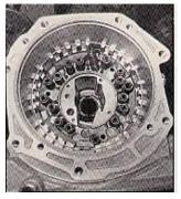
6. Assemble the output shaft and install the direct clutch sprag. If you remove the side washer on the sprag, you'll notice a shoulder on one side of the sprag. Make sure this shoulder is on the output side of the shaft when installing the sprag on the shaft.
