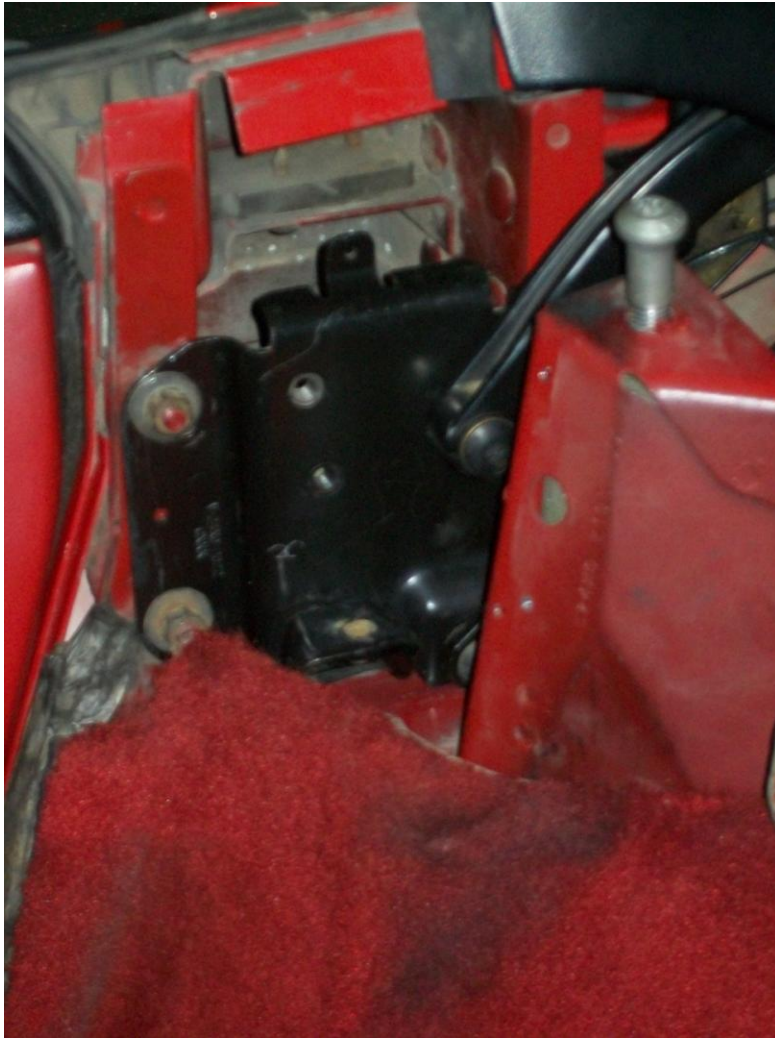
Figure 13 - Swapped out 89-96 B Pillar bracket for attaching hardtop
