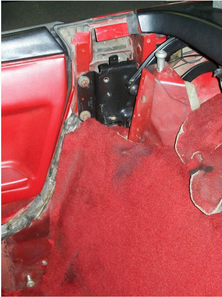
Figure 10 - Swapped out 89-96 B Pillar bracket for attaching hardtop
