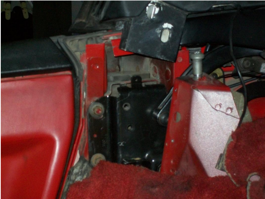
Figure 20 - Hardtop sitting on car. Note location of mounting bracket at B Pillar
