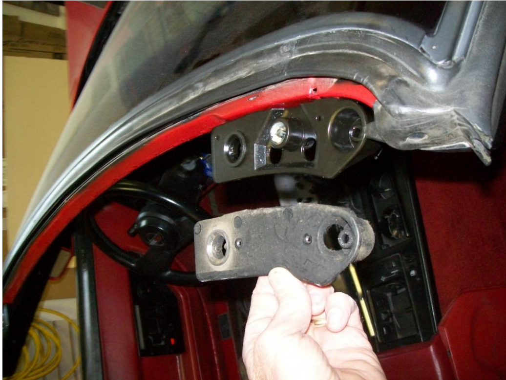
Figure 14 – Change out windshield header brackets for attaching hardtop. 89-96 bracket is attached and holding original 87 bracket for comparison.
