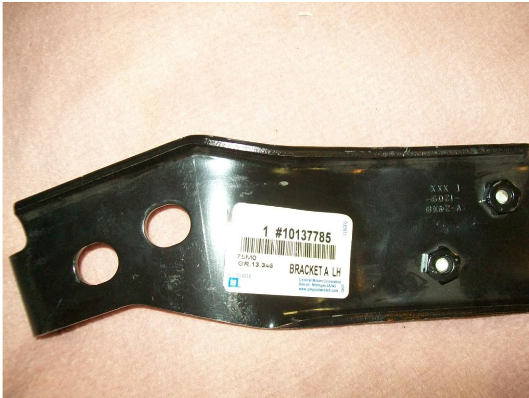
Figure 5 - Backside of Factory Hardtop bracket for attaching Hardtop to B pillar
