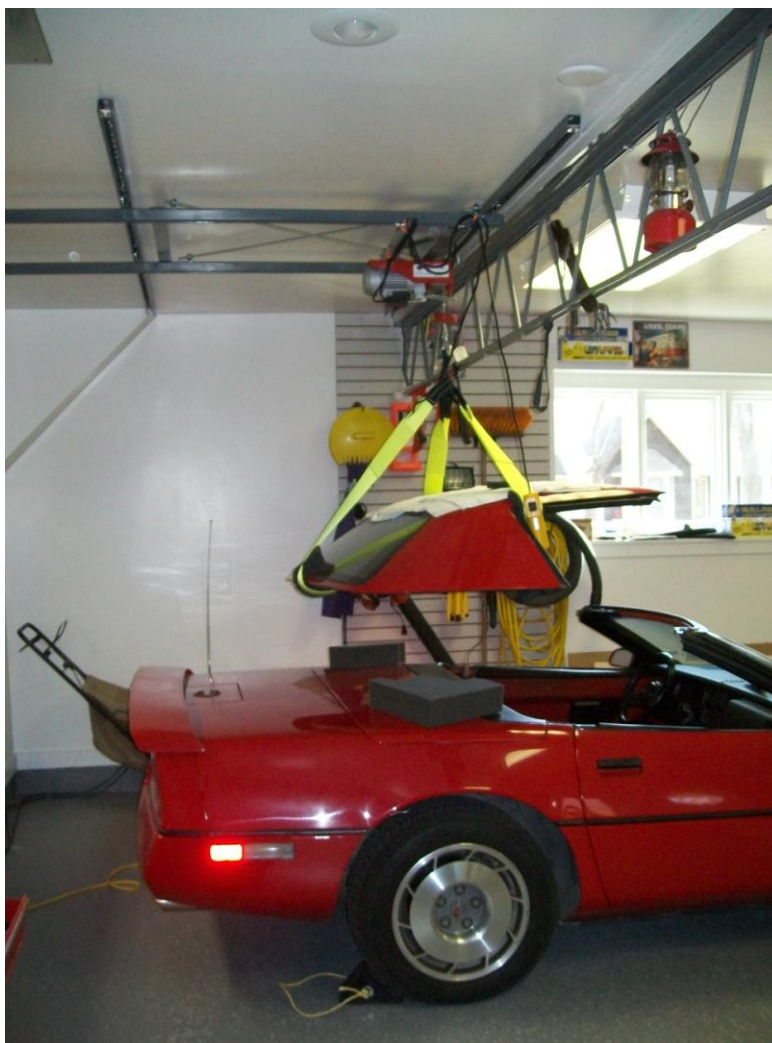
Figure 17 - Preparing to lower hardtop onto car
