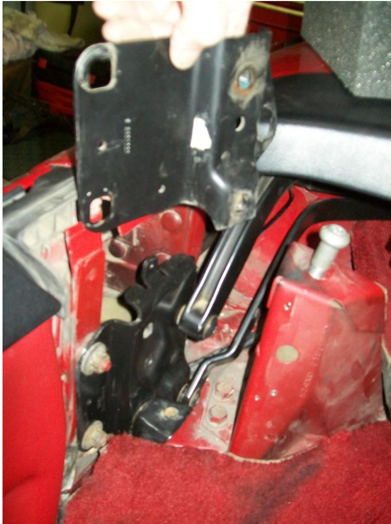
Figure 9 - Swapped out 89-96 B Pillar bracket for attaching hardtop
