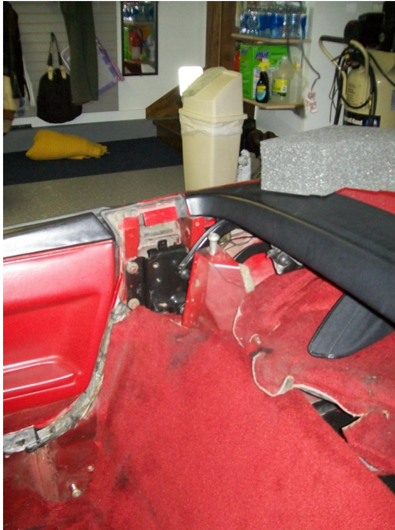
Figure 11 - Swapped out 89-96 B Pillar bracket for attaching hardtop
