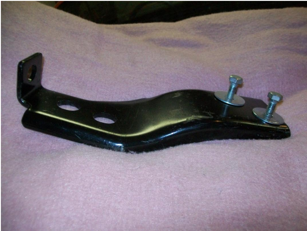
Figure 4 - Factory Hardtop bracket for attaching Hardtop to B pillar
