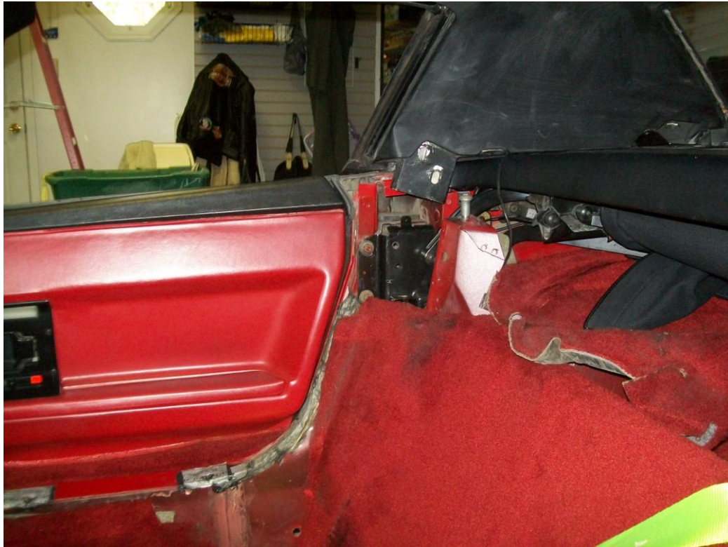
Figure 21 - Hardtop sitting on car. Note location of mounting bracket at B Pillar
