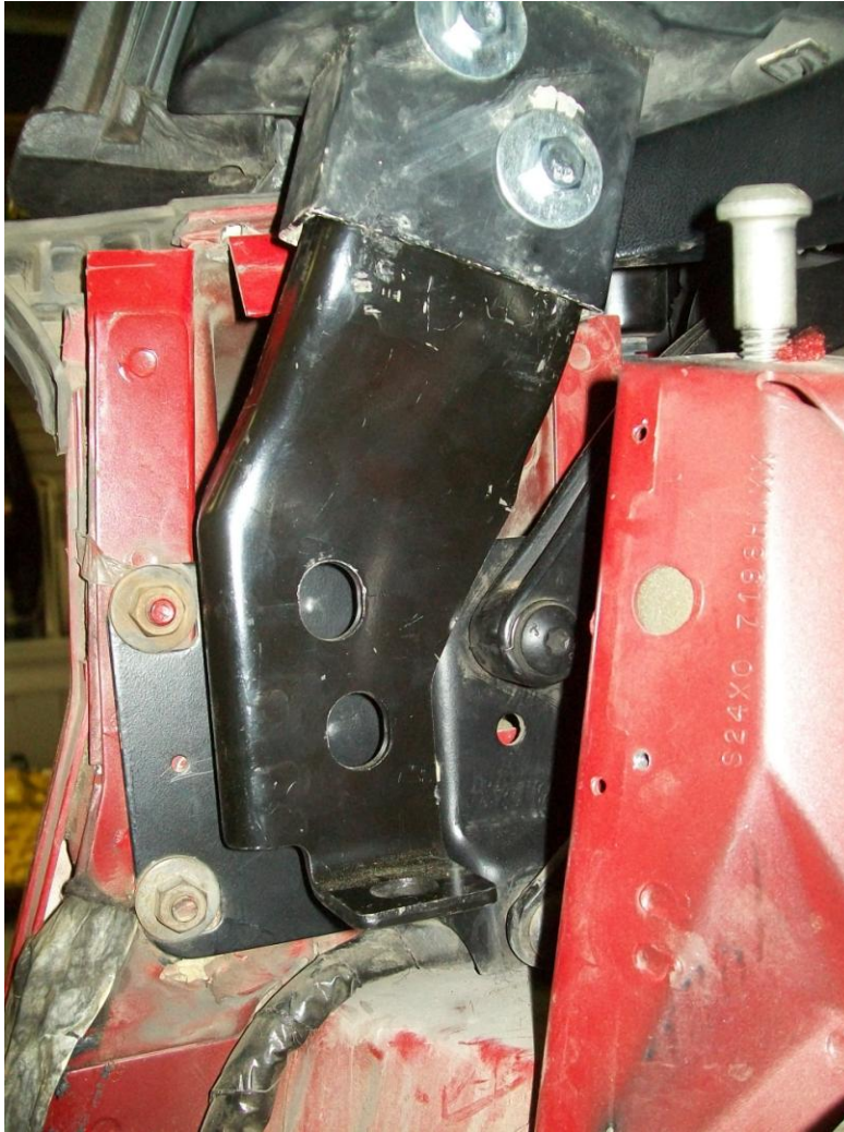
Figure 6 - Stock 84 – 88 B-pillar bracket on my 87 convertible does not allow for bolt-up of hardtop bracket
