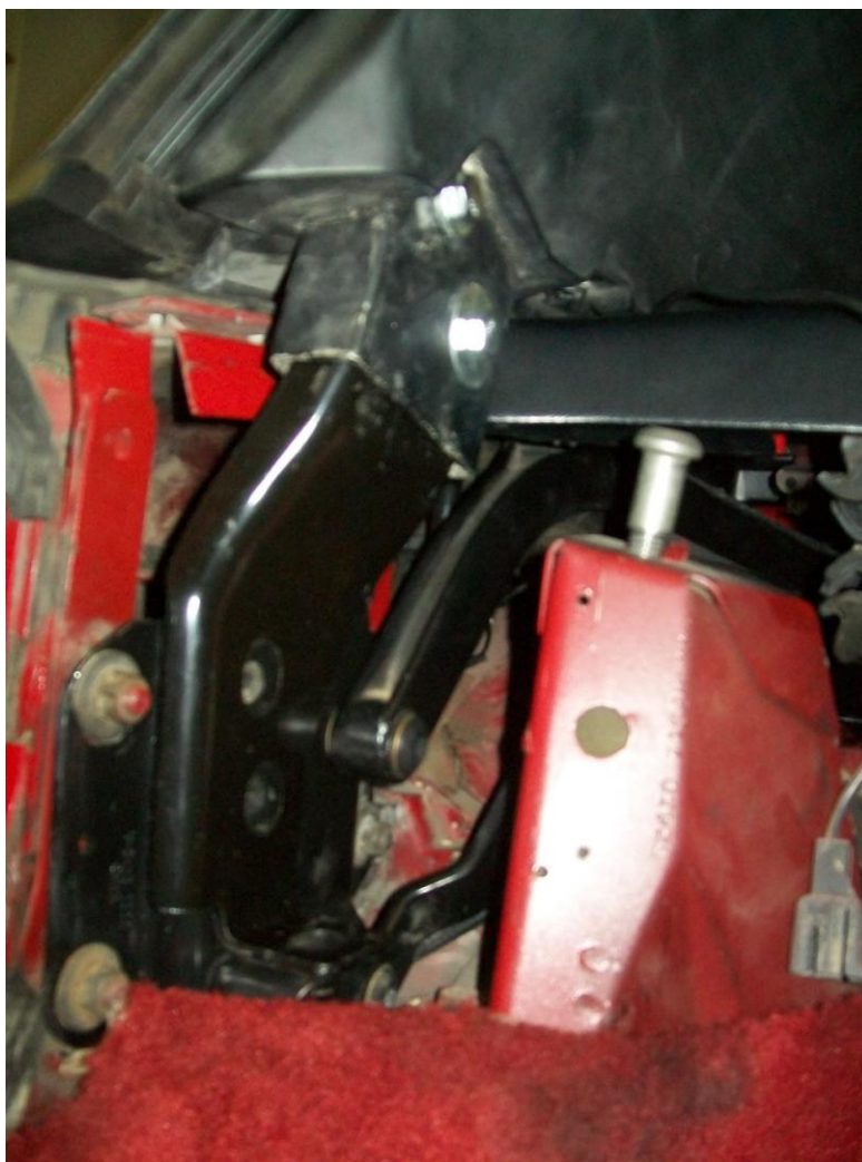
Figure 22 - Hardtop mounting bracket installed for connection to B Pillar pivot arm bracket
