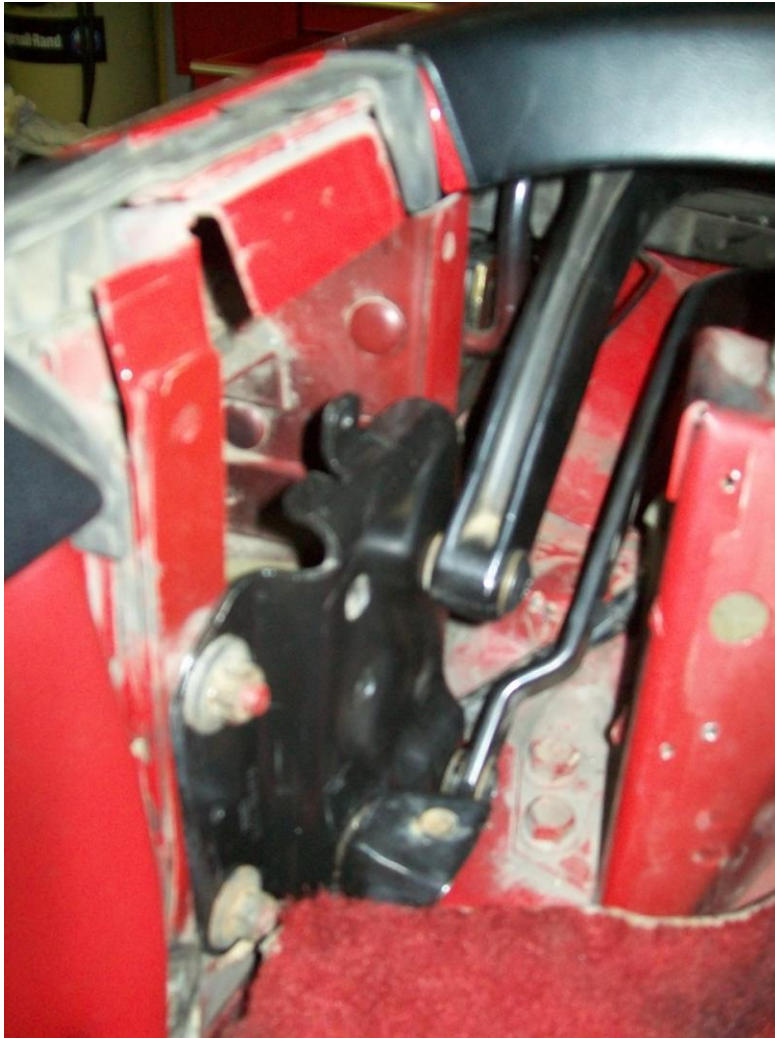
Figure 12 - Swapped out 89-96 B Pillar bracket for attaching hardtop
