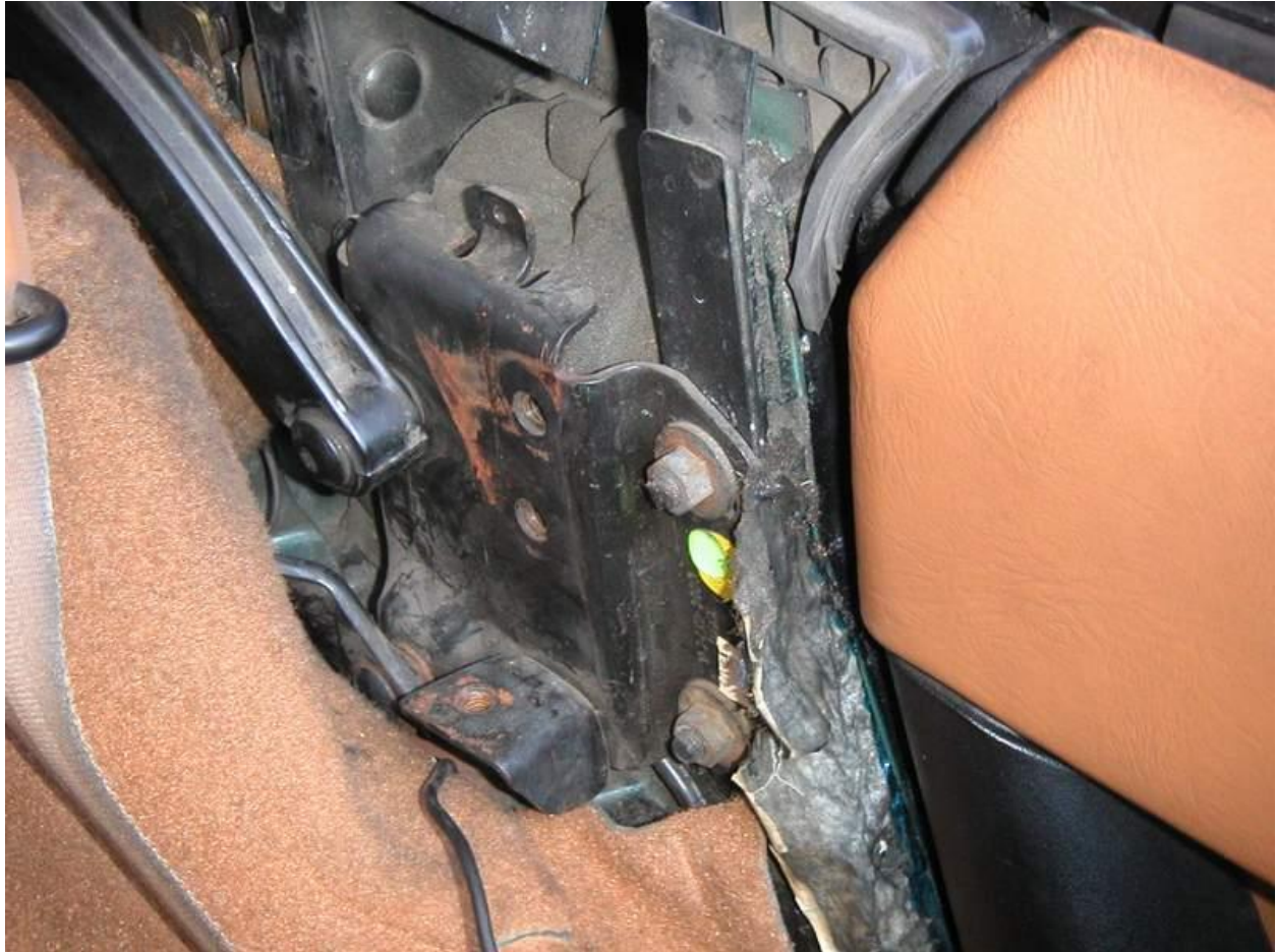
Figure 8 - Picture from Internet of 89-96 B Pillar bracket for attaching hardtop
