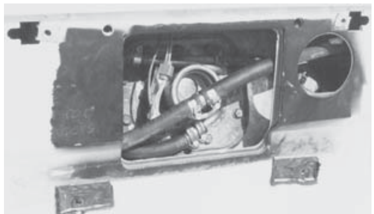
Fuel Filler Neck, Fuel Line and Wiring Connection
